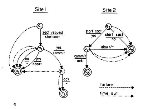
Figure 7. The extended two-phase protocol of figure 5 augmented with failure and time-out transitions according to rules 1 and 2.
