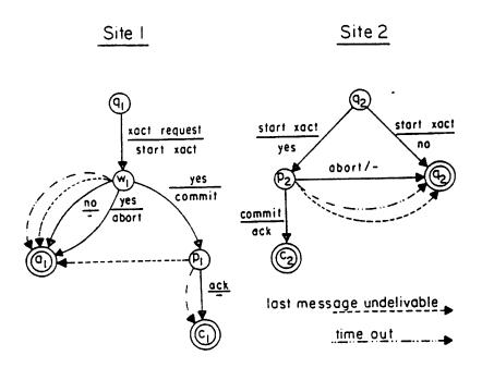
Figure 8. The extended two-phase commit protocol (of figure 5) augmented with time-out transitions and transitions on undeliverable messages according to rules 3 and 4.
