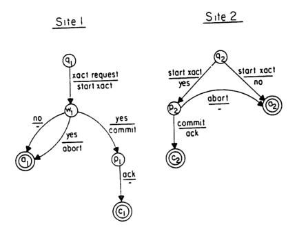
Figure 5. Two-phase commit protocol extended with an ack message.
