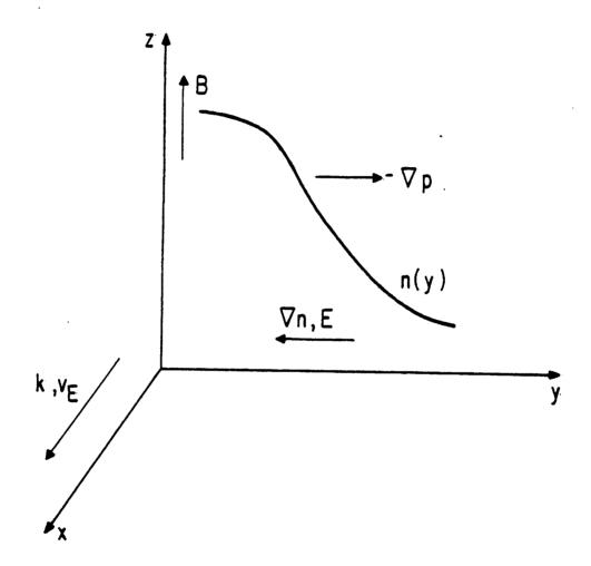
FIG. 1 Slab coordinates for lower-hybrid drift instability.
