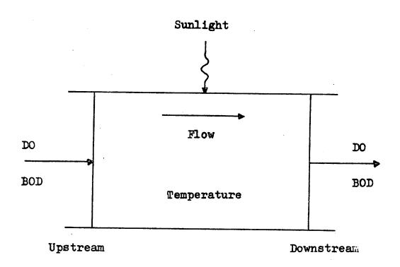
Figure 4. Schematic of the river system
