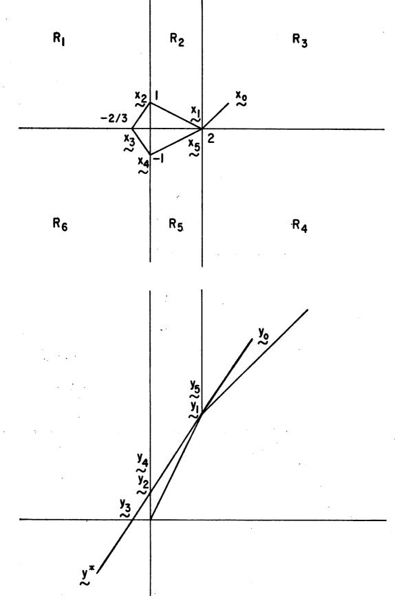
Fig. 7. Cyclic solution curve through a corner.
