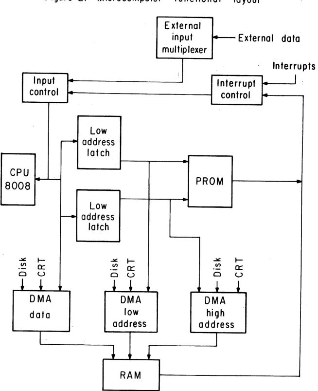
Figure 2. Microcomputer functional layout
