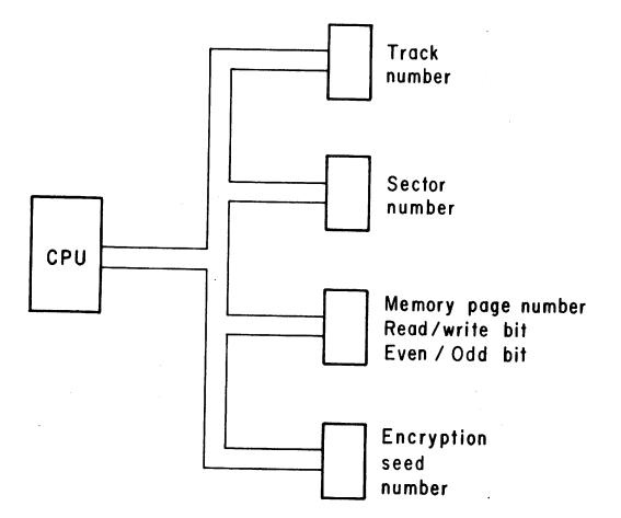
Figure 6. I/O validation and gatekeeper circuitry
