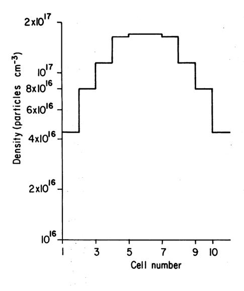
Fig. 10 Density profile for a 10 cell system with M = 5 and S =  $5 \times 10^{23}$  particles cm<sup>-2</sup> sec<sup>-1</sup>.
