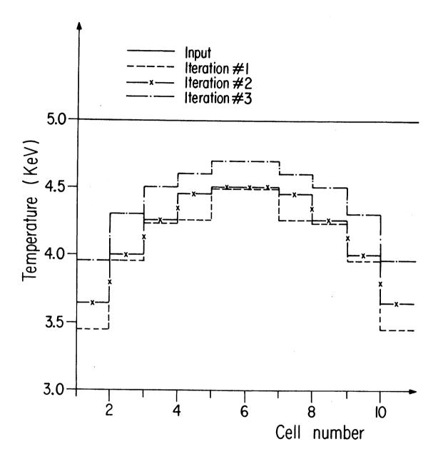
Fig. 9 Cell temperatures in a multiple mirror system;  $S = 2.6 \cdot 10^{23}$  particles cm<sup>-2</sup> sec<sup>-1</sup>.
