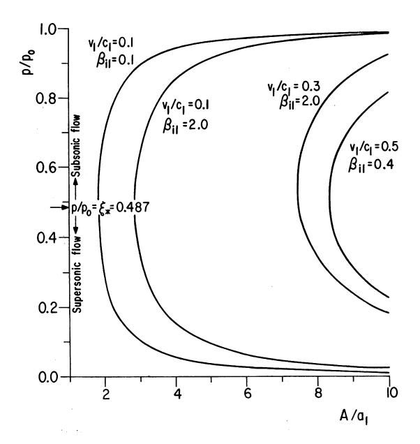
Fig. 5 Pressure variation in a converging-diverging magnetic nozzle  $A_1/a_1 = 10 \ , \ \gamma = 5/3 \ .$
