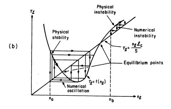
Fig. 11b Physical stability with numerical oscillation and physical and numerical instability.
