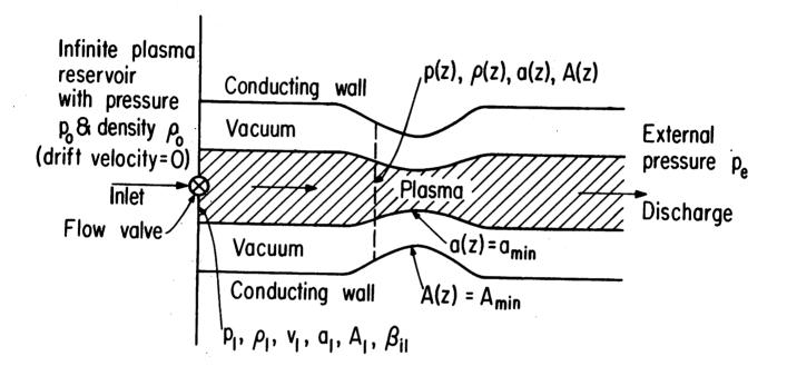
Fig. 4 A magnetic converging-diverging nozzle.
