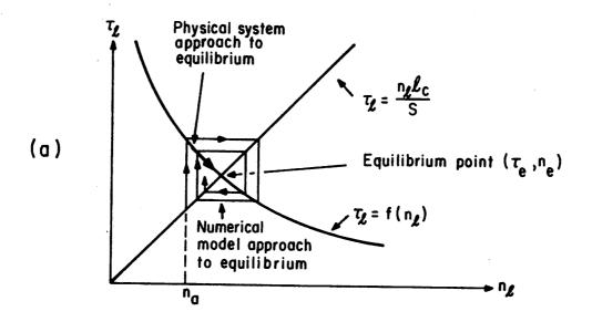
Fig. 11a Physical and numerical stability
