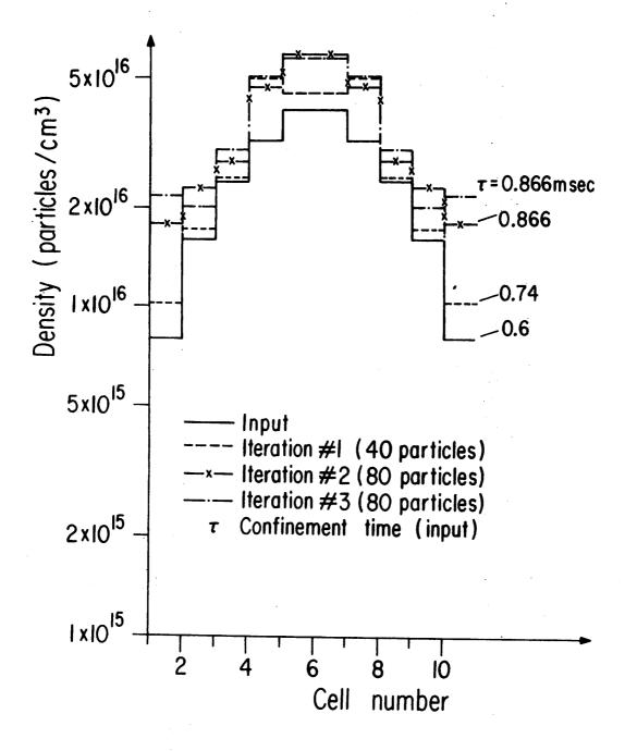
Fig. 8 Cell densities in a multiple mirror system;  $S = 2.6 \cdot 10^{23}$ particles cm<sup>-2</sup> sec<sup>-1</sup>.
