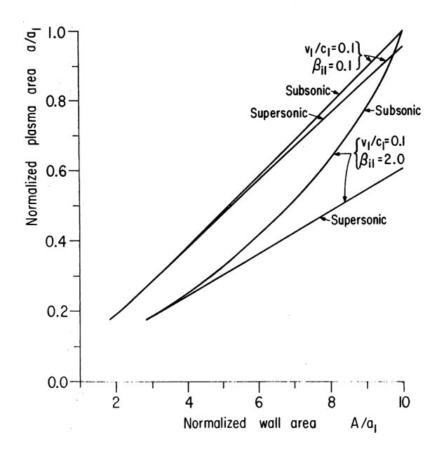
Fig. 6 Variation of plasma area with wall area for  $A_1/a_1 = 10$ ,  $\gamma = 5/3$ .
