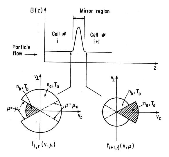
Fig. 3 Schematic representation of the distribution function on either side of a collisionless mirror
