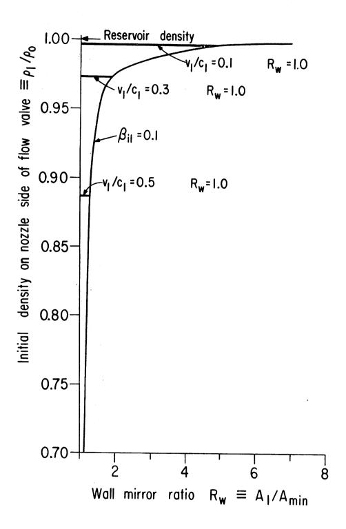
Fig. 7 Variation of initial density with wall mirror ratio (constant mass flow W).
