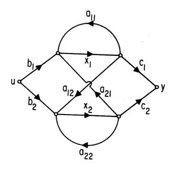
Fig. 2. A scalar signal flow graph which realizes a second-order transfer function.
