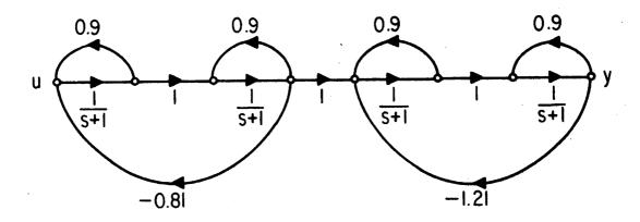
Fig. 5. Initial design of a 4th order system.
