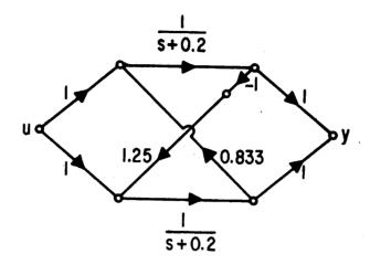
Fig. 3a. The signal flow graph representation of the circuit in Fig. 3b.
