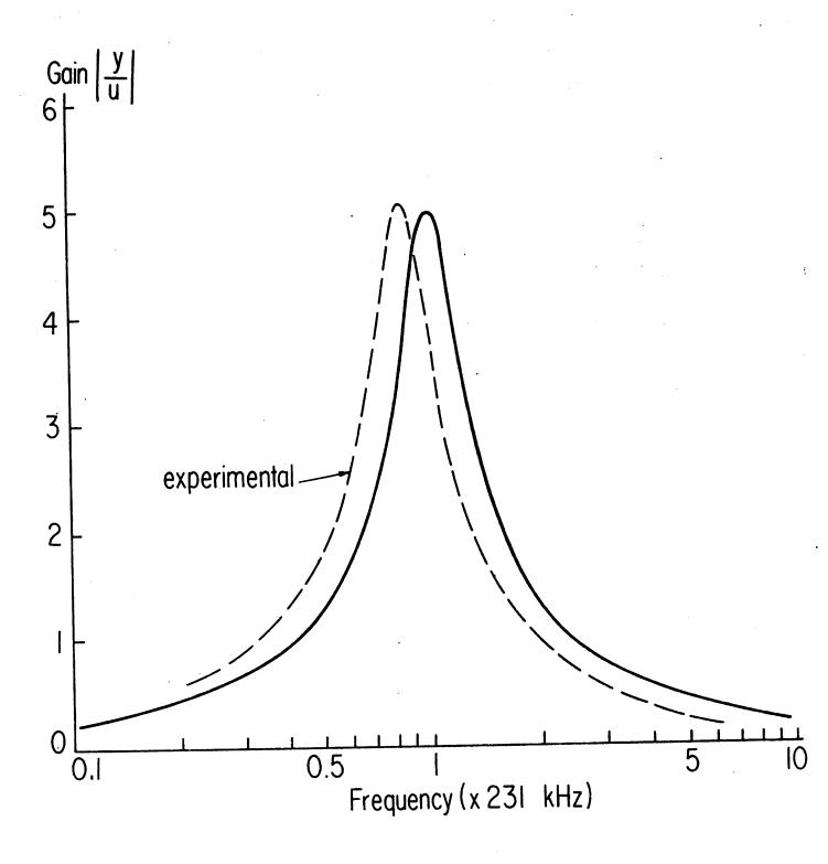
Fig. 4. Measured and designed frequence responses for the circuit in Fig. 3b.
