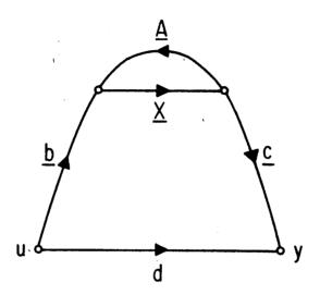
Fig. 1. A general multiple loop feedback configuration which is represented by a vector signal flow graph. u is the scalar input, y is the scalar output, and X is an n x n diagonal matrix whose individual elements represent n active stages.
