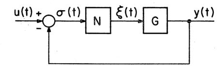
Fig. 1. Nonlinear feedback system.
