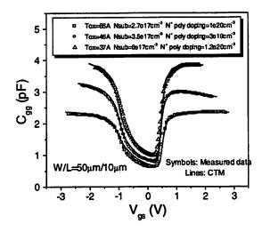
Figure 7. CTM verified with measured NMOSFET Cgg for various oxide thickness, substrate and polysilicon gate doping concentrations.
