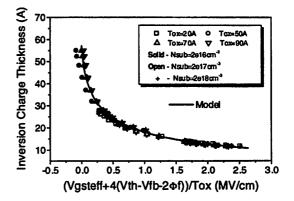
Figure 4. For all *Tox* and *Nsub*, modeled inversion charge thickness agrees with numerical quantum simulations.
