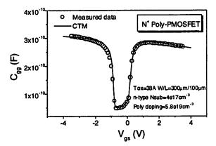
Figure 8. Measured and CTM modeled Cgg of N<sup>+</sup>-poly (buried-channel) PMOSFET. Gate depletion occuring in the accumulation region is correctly modeled.
