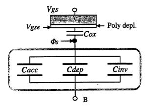
Figure 2. Charge-thickness capacitance concept in this model. *Vgse* accounts for poly-depletion.
