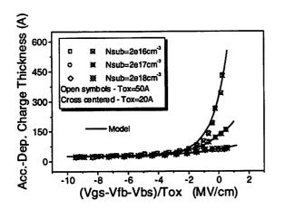
Figure 3. For all Tox and Nsub, modeled charge thickness agrees with numerical quantum simulations throughout accumulation and depletion regions.
