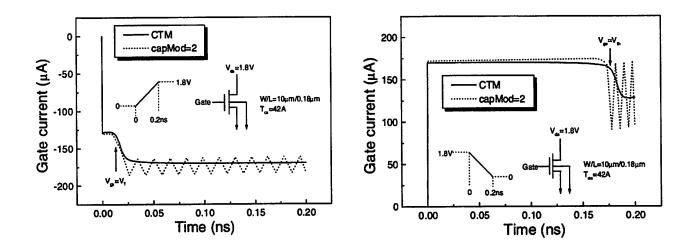
Figure 13. Comparison of gate currents in turn-on and turn-off transients between CTM and BSIM3v3.1 capmod=2 for an NMOSFET with  $W/L=10\mu m/0.18\mu m$  and  $T_{ar}=42A$ . The absence of the gate current oscillation in CTM helps convergence.
