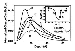
Figure 1. Charge distributions from numerical quantum simulations show significant charge thickness at various bias conditions shown in the inset.
