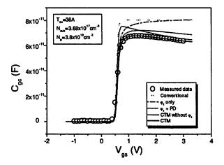
Figure 10. Measured and modeled gate-to-channel capacitance  $C_{gc}$  of an NMOSFET with different physical effects considered in simulation.  $T_{ox} = 36$ A,  $W/L = 100 \mu m/100 \mu m$ ,  $N_p = 3.8 \times 10^{19} \text{ cm}^{-3}$  and  $N_{sub} = 3.68 \times 10^{17} \text{ cm}^{-3}$ . PD stands for Polysilicon Depletion.
