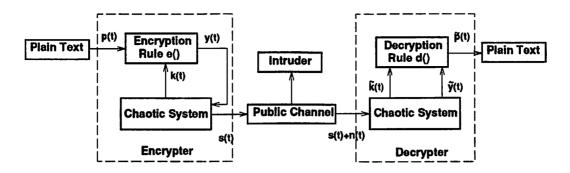
Figure 1: Block diagram of the chaotic cryptosystem.
