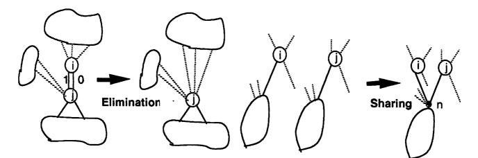
Fig.8 Two basic procedures to reduce BDD. The sneak-path free nature is demonstrated by using this figure.
