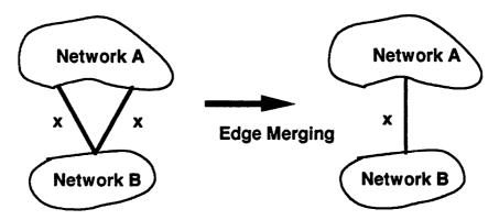
Fig.7 Edge-Merging technique.
