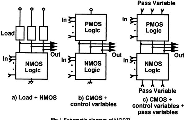
Fig.1 Schematic diagram of MOSTL
