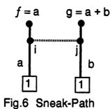
A very powerful transformation in constructing MOSTL is 'edge-merging' as shown in Fig.7. The essence of the edge-merging is to merge two edges with one node common controlled by the same variable into one edge. Other than the BDD based method described above, this edge-merging seems promising. The drawback of the edge-merging, however, is the creation of sneak-path.
