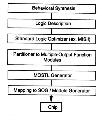
Fig.9 MOSTL generator incorporated in a design system
