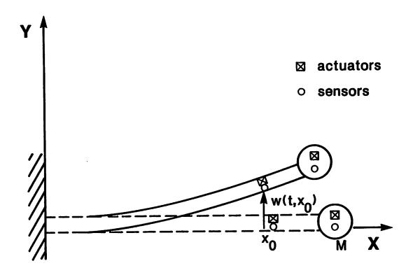
Figure 2: Planar bending motion of a flexible beam.
