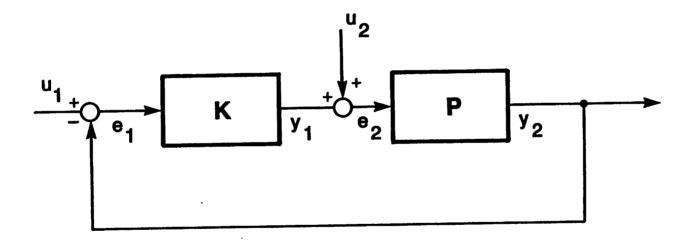
Figure 1: The feedback system S(P,K).
