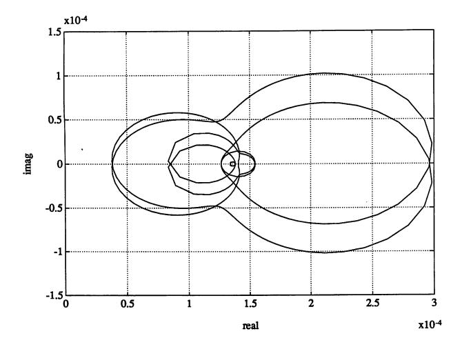
Figure 4: Modified Nyquist diagram for the stabilized system.
