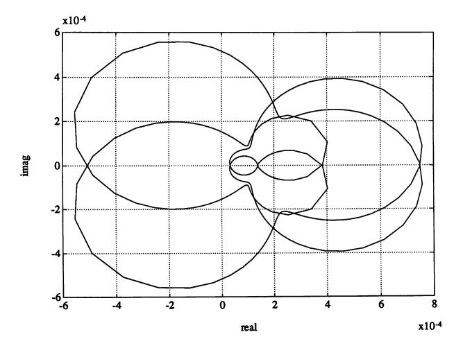
Figure 3: Modified Nyquist diagram (initial design).
