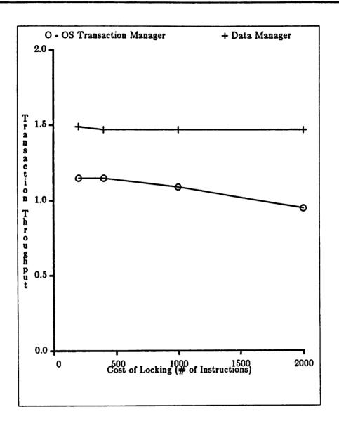
Figure 3: Effect of cost of locking on throughput
