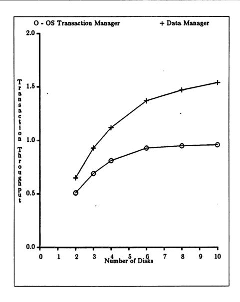
Figure 4: Effect of increasing disks on throughput
