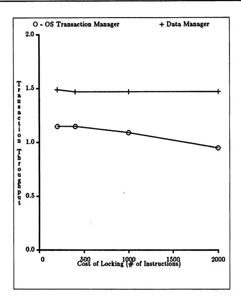
Figure 5: Effect of cost of locking on throughput
