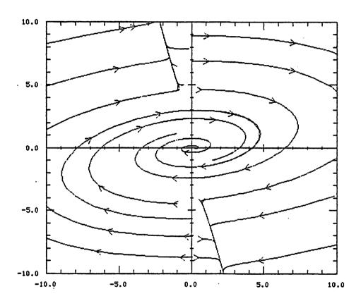
Figure 2. Phase portrait of center manifold system of the stabilized system.
