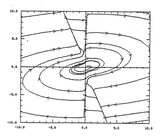
Figure 3. Phase portrait on the invariant manifold of the perturbed system.
