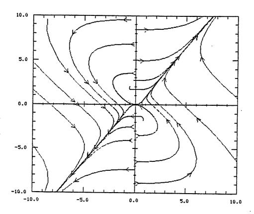
Figure 1. Phase portrait of center manifold system of the unstable system.
