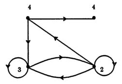
Fig. 5.1 - Possible transitions when waiting for a lock
