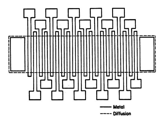
Figure 6  $Measurement \ technique \ for \ determining \ contact \ end \\ resistance, \ R_E, \ as \ a \ ratio \ of \ v_2 \ to \ i_1^{26}$
