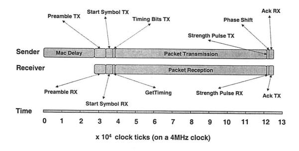
Figure 1: Timing Diagram of Network Send/Receive
