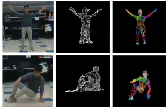
Figure 1. Model fitted to various observed posture. Left is the RGB camera input. Center is the observed depth camera input as a point cloud. Right is the estimated deformable model pose.
