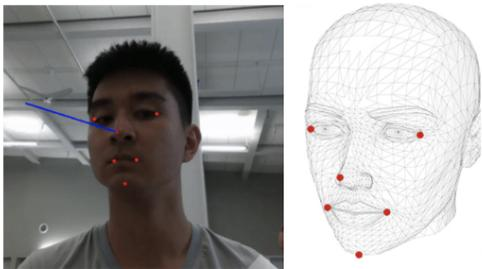
Figure 5. Positions of 6 corresponding facial landmarks are computed both on the RGB and synthetic face mesh. We solve 2D-3D correspondence problem[28] to recover the head direction from the RGB view,
