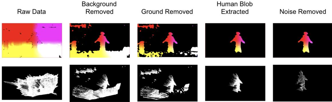
Figure 3. The raw image is acquired from the depth camera the human point cloud is extracted through the preprocessing procedure. First, the background and ground plane are removed. Next, small blobs are the human are removed. Finally, the data is downsampled, averaged, and outlier points are removed.
