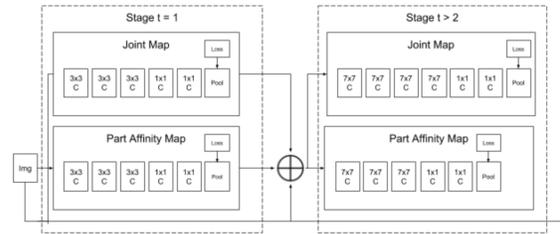
Figure 4. Two stage neural network proposed by OpenPose. Modification are made to the part affinity map to use less convolutional layers since our tracking is constrained to a single person.
