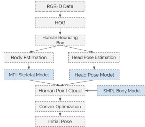
Figure 2. System pipeline that takes in a single view RGB-D and fits an initial pose to the observed data. In this pipeline, three models (MPII Skeletal Model, Head Pose Model, and SMPL Body Model) are built and fused via a convex optimization.
