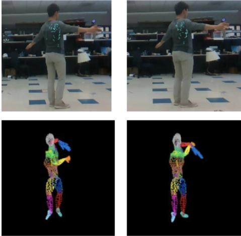
Figure 7. Poses that introduces significant self occlusion are problematic for the current approach. We hypothesis this may be due excessive sensor noise in these fast moving cases
