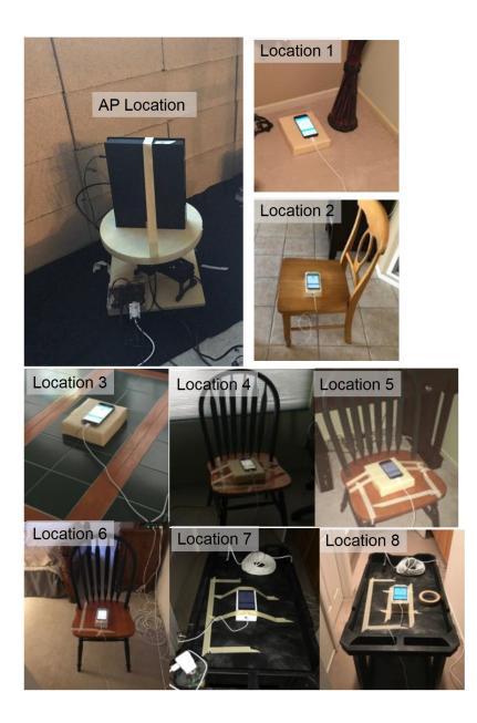
Figure 5.11: Access point turntable setup and client test locations.
