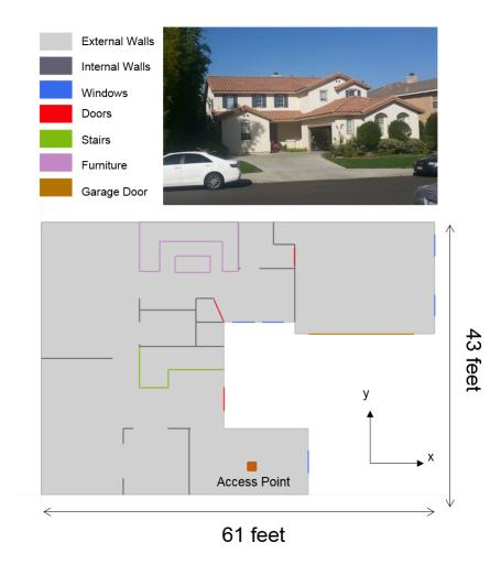
Figure 5.3: First floor layout of the test hose including simulation materials.
