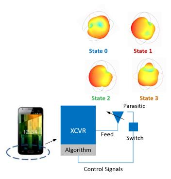
Figure 2.7: System architecture of a modal adaptive antenna system. The system contains a modal antenna structure, a switch, and an algorithm that changes the state of the switch and antenna based on real-time channel state feedback from the transceiver.
