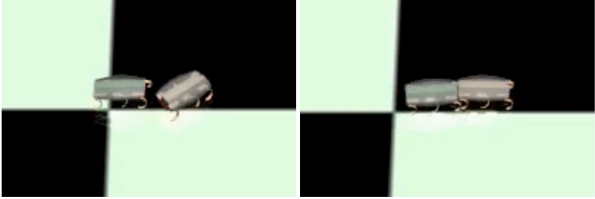
Figure 4.3: The magnets attract and pull two robots together in the simulation.
