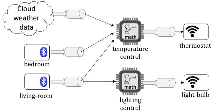
Figure 5: An example building-automation solution, where physical sensors and actuators are represented by logs to applications. Each application can have multiple input/output logs, including those representing external data sources. Each sensor log can be subscribed by multiple applications as well.
