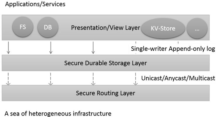
Figure 2: A refactoring of interfaces for a cleaner design of a widely distributed system (see § 1.2). A secure single-writer append-only log interface acts as a bridge between the “presentation/view layer” and the “secure durable storage layer”. Similarly, the “secure durable storage layer” utilizes unicast/anycast/multicast to utilize the “secure routing layer underneath”. See § 1.2 for details.
