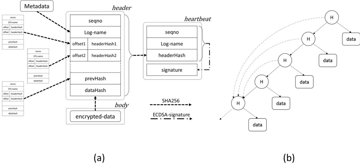
Figure 6: (a) Record structure demonstrating record-header, body and heartbeat. (b) Without hash-pointers (*offset*, *headerHash*), the records in a log make a very skewed Merkle tree (essentially a hash-chain). Hash-pointers include additional links and transform the Merkle tree to a Directed Acyclic Graph (DAG).
