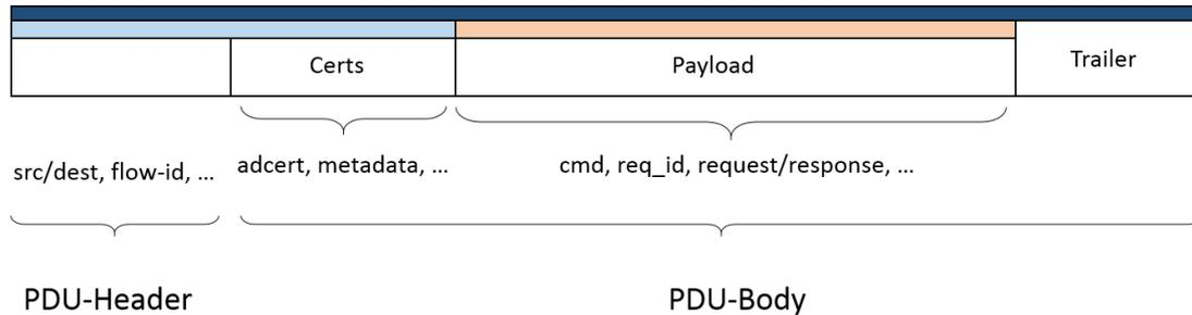
Figure 8: GDP protocol PDU. PDUs are split in two parts: a *PDU header* and a *PDU body*. PDU Header primarily contains ‘source’ and ‘destination’ information and is used by the GDP-network to route messages. The PDU body is split into three parts: *certs*, *payload* and *trailer*. *Certs* contains certificates and metadatas for key-exchange; *payload* contains the actual request/response to/from a log-server; *trailer* contains an HMAC (or a signature) from the log-server.
