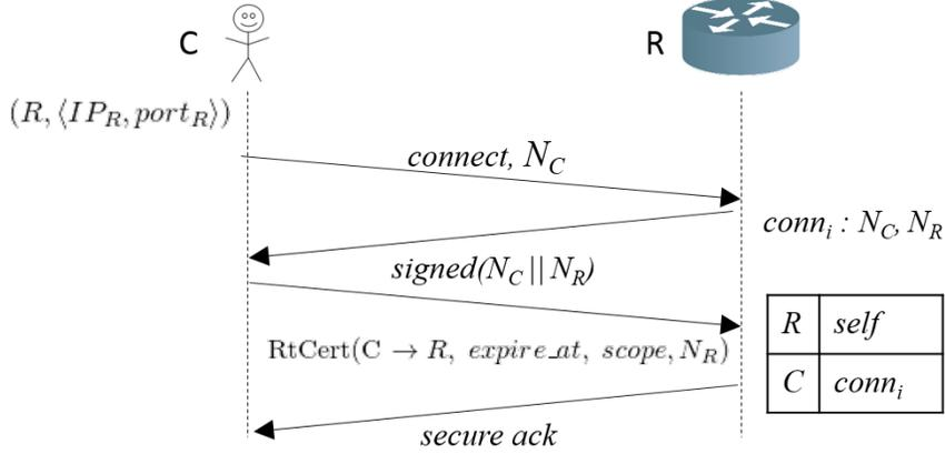
Figure 9: Local advertising process: A client  $C$  sends a routing certificate to a router  $R$ . After certificate validation,  $R$  updates its local forwarding table.
