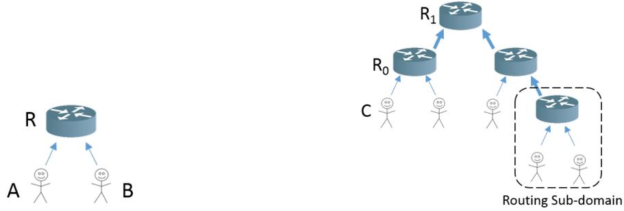
(a) A standalone router  $R$  that can securely route messages between clients  $A$  and  $B$
