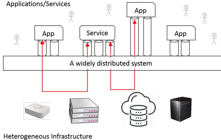
Figure 1: A widely distributed system spread over heterogeneous infrastructure that provides a uniform *platform* for applications (see § 1.1).
