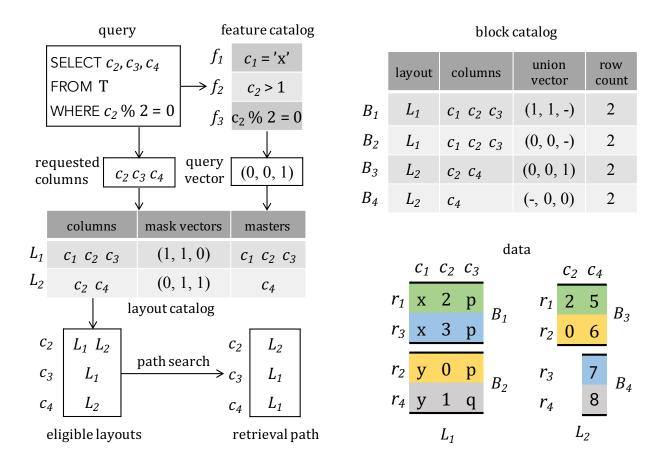
Figure 5.6: Example of Query Processing in GSOP-R.
