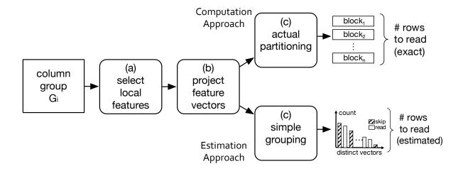
Figure 4.5: Computation Approach vs. Estimation Approach for GSOP
