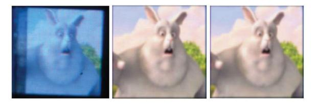
Figure 8.8: Left: Physical Experiment, Center: Ray Optics Simulation, Right: Wave Optics Simulation
