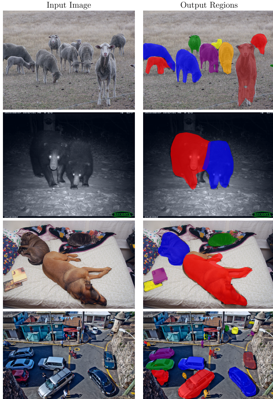
Figure 4.7: Output visualization. For each of these images from the validation set, we show the closest matching predicted region to each ground truth region (in terms of I/U). (Note that some objects are correctly predicted, but no region is shown because a label does not exist in the ground truth.) Note the ability to find occluded objects, to separate objects without sharp boundaries (second example), and to find small objects in cluttered scenes (without neglecting large objects).
