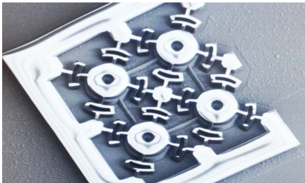
Figure 6.4: SEM inspection of hard-baked 3- \mu\text{m} -thick photoresist after patterning and before etching the top electrode.
