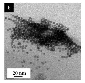
Figure 3.7: TEM analysis of the drop-casted nanocomposite films. These images show that nanoparticles are dispersed in form of clusters in the SU-8 polymer matrix.
