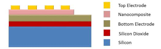
Figure 4.1: Cross-sectional schematic of the capacitor structure in metal insulator metal (MIM) configuration
