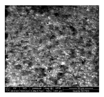
Figure 3.2: SEM image of the top surface of drop-casted nanocomposite film (sample-1). As evident from the presence of microbubbles and voids, a porous nanocomposite film is obtained.
