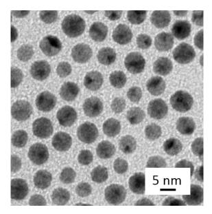
Figure 3.6: TEM image of dodecanethiol functionalized gold nanoparticles
