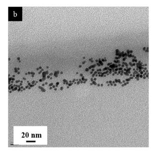
Figure 3.9: TEM images from the various regions of the spin-coated nanocomposite film. These images suggest that nanoparticles have agglomerated in the SU-8 polymer for spin-coated nanocomposite films as well.
