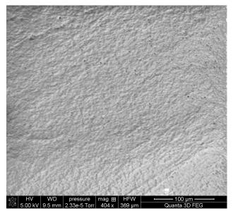
Figure 3.4: SEM image of the top surface of the spin-coated nanocomposite film (sample-3). There are few voids but overall a dense film is obtained.
