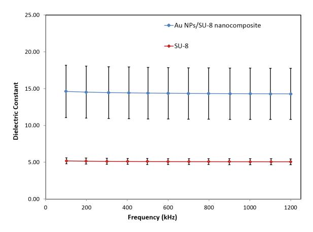
Figure 4.3: Dielectric constant of nanocomposite and SU-8 material from 100 KHz to 1.2 MHz. Measured dielectric constant values for the nanocomposite samples are higher than the SU-8 only samples.
