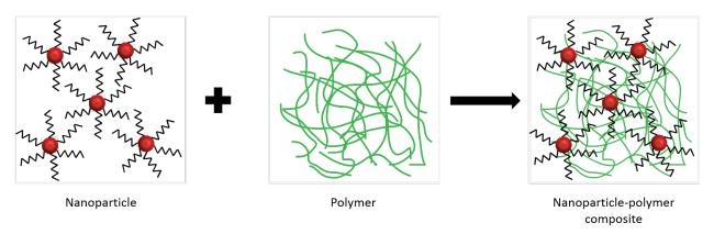
Figure 2.3: *Ex situ* method of polymer nanocomposite material synthesis. In this technique, nanoparticle and polymer components are synthesized separately and then blended to prepare the nanocomposite material.
