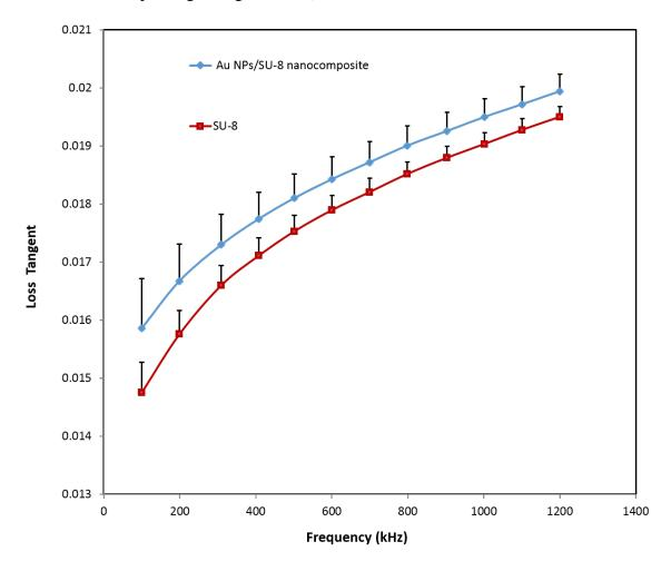
Figure 4.4: Measurement of loss tangent values for nanocomposite and SU-8 only samples.
