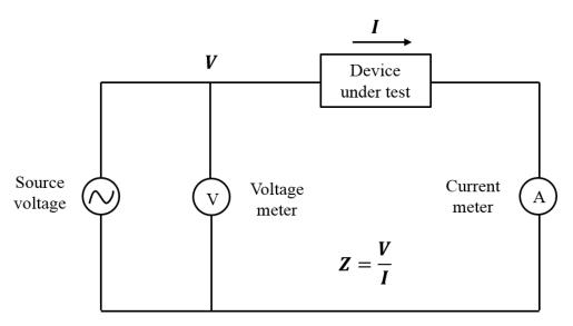
Figure 4.2: Equivalent circuit diagram of the dielectric spectroscopy set-up
