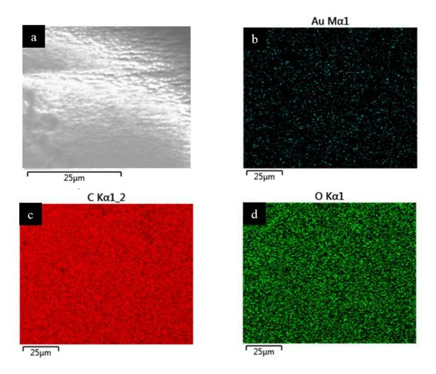
Figure 3.5: EDX analysis of the gold nanoparticle/SU-8 polymer composite material. Figure 3.5 (a) corresponds to the SEM image of the top surface of nanocomposite film. The individual elemental maps are shown in Figure 3.5 (b-d). These maps reveal that C, O and Au are the elemental constituents of the nanocomposite film. Further, the elemental map of Au qualitatively suggests a homogeneous dispersion of gold nanoparticles in the polymer matrix.
