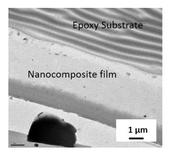
Figure 3.8: Cross-section of the spin-coated nanocomposite film.
