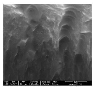
Figure 3.3: Cross-section of the nanocomposite film obtained from sample-2. Unlike sample-1, there are no voids through the nanocomposite film, but a thicker film is obtained ( $\sim 65 \,\mu m$ ).
