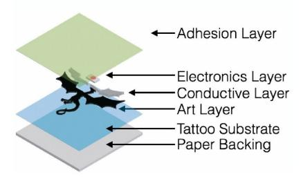
Figure 1.1 Components of Skintillates
