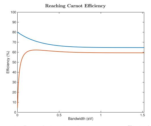
Figure 5.12: The efficiency of a thermophotovoltaic system assuming 100% back reflectivity and  $\eta_{ext} = 100\%$ , as a function of the bandwidth above the bandgap that is transmitted to the cell (blue line) and assuming 99% back reflectivity (red line).
