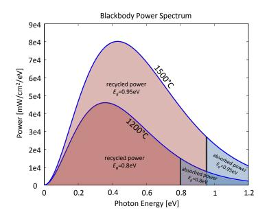
Figure 5.7: The blackbody power spectrum, for blackbody sources at  $1500^{\circ}C$  and  $1200^{\circ}C$ . For a 0.8eV bandgap cell and a  $1200^{\circ}C$  source, the power absorbed by the solar cell is indicated by the blue region, and the power recycled back to the hot source is indicated by the red region. Similarly for a 0.95eV bandgap cell and a  $1500^{\circ}C$  source, the regions of recycled power and absorbed photon are highlighted in red and blue, respectively.
