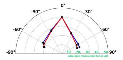
Figure 4.14: The absorption enhancement factor (AE) averaged over frequency and polarization, as a function of incident angle  $\theta$  in the xz plane (blue) and the yz plane (red).
