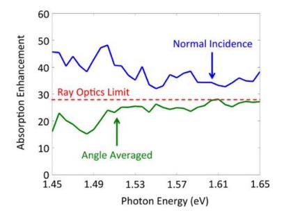
Figure 4.34: Angle averaged and normal incidence performance for the constrained height texture in Fig. 4.33.
