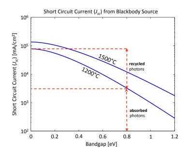
Figure 5.8: The short circuit current (Jsc) as a function of bandgap, for blackbody sources at  $1500^{\circ}C$  and  $1200^{\circ}C$ . For a 0.8 eV bandgap cell and a  $1200^{\circ}C$  hot source, 4% of the photons emitted by the blackbody are above bandgap and thus absorbed by the photovoltaic cell, while 96% are recycled back to the hot source, as indicated by the red dashed lines.
