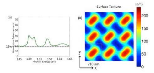
Figure 4.21: (a) The final absorption enhancement as a function of frequency and (b) a topdown view of the surface texture, showing broken mirror symmetry, from almost symmetric initial conditions seen in Fig. 4.20.
