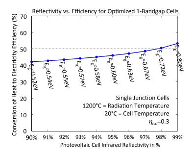
Figure 5.5: The efficiency as a function of photovoltaic cell infrared reflectivity for single junction cells. The source radiation temperature is  $1200^{\circ}C$ , the cell temperature is  $20^{\circ}C$ , and  $\eta_{ext} = 0.3$ .
