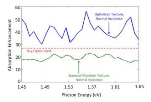
Figure 4.30: The absorption enhancement as a function of frequency at normal incidence for the optimized texture from Fig. 4.15(b) (blue) compared with the median random texture with 2300 nm periodicity from Fig. 4.29 (green). Lines are averaged over the two orthogonal polarizations.
