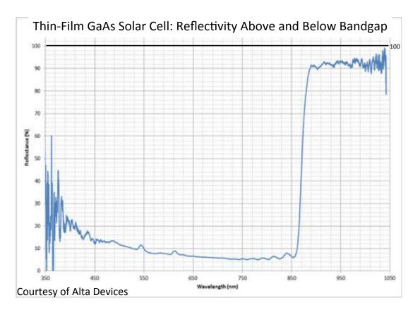
Figure 5.2: Reflectivity of a standard production GaAs solar cell from Alta Devices Inc. (The world record cell had even higher sub-bandgap reflectivity, 98%.) Achieving the same step function response, in an InGaAs alloy, would be ideal for thermophotovoltaics.
