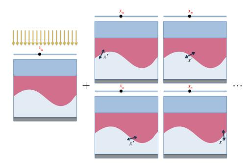
Figure 4.9: Without the adjoint method, we needed n + 1 simulations in order to calculate the Shape Derivative.
