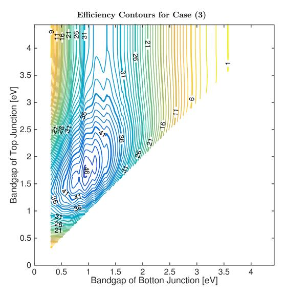
Figure 3.7: The efficiencies as a function of top and bottom bandgap for Case (3), a dual junction cell with an air gap intermediate mirror and perfect back mirror.
