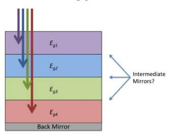
Figure 3.1: Bandgaps of different materials are placed in a stack, from largest bandgap on top to smallest on the bottom in a multi-bandgap cell. The question arises, how do we design intermediate mirrors that reflect internally luminescent photons without impeding the transmission of externally incident photons?
