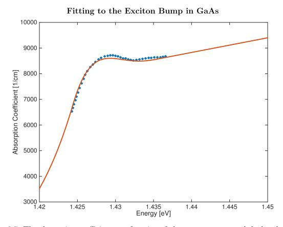
Figure 2.7: The absorption coefficient as a function of photon energy, around the bandedge of GaAs. The blue crosses represent the data from [17], showing a bump around the bandedge due to absorption at the exciton energy. The absorption coefficient fit described in [5] ignores this exciton bump. We use the fit in [5], except at the bandedge, where we model the exciton bump with a fourth degree polynomial. The red line shows our fit.
