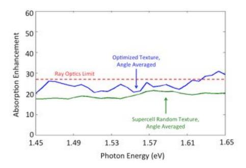
Figure 4.31: The absorption enhancement as a function of frequency, angle averaged, for the optimized texture from Fig. 4.15(b) (blue) compared with the median random texture with 2300 nm periodicity from Fig. 4.29 (green).
