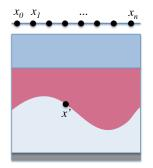
Figure 4.4: We can derive the change in figure of merit due to adding a piece of material at a particular x'.
