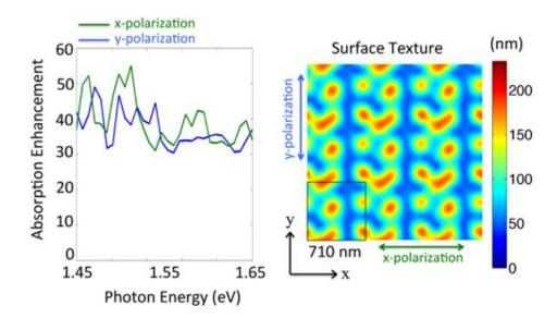
Figure 4.33: Final texture for the optimization with a height amplitude constraint and absorption enhancement for normal incidence light.
