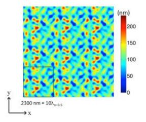
Figure 4.29: A top-down view of the surface texture, for the randomly generated texture with periodicity of 2300 nm =  $10\lambda_n = 3.5$ , with median Figure of Merit (minimum absorption enhancement).
