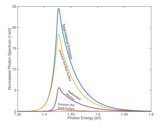
Figure 2.6: The breakdown of internal photons in a GaAs cell, grown on a substrate for a 100 nm thick cell. The spectrum is shown for total internal emission, normalized to unity (blue). Of the total internal spectrum, the fraction of photons reabsorbed by the cell (purple), photons escaping out the front surface (red), and photons emitted in the substrate (yellow), are shown.
