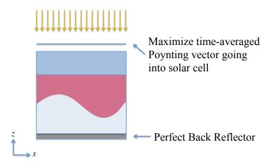
Figure 4.2: We want to increase the absorption, and equivalently, the Poynting vector into the solar cell material by optimizing a periodic surface texture function.
