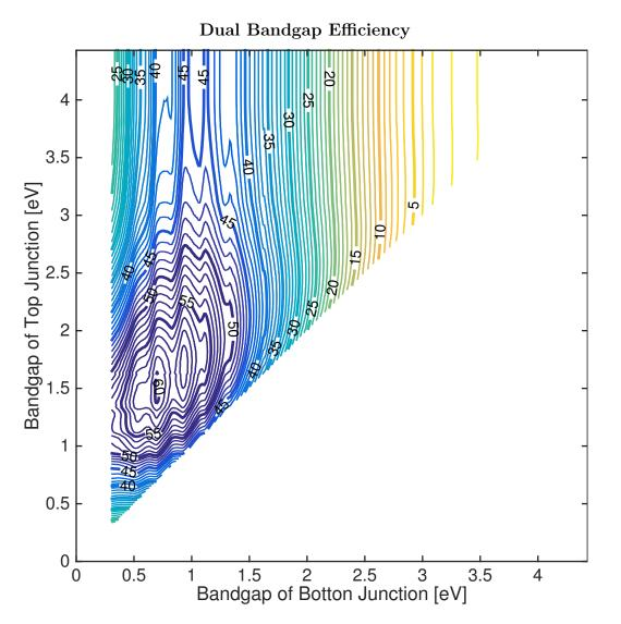
Figure 6.2: Efficiency of dual bandgap solar cells under maximum concentration.
