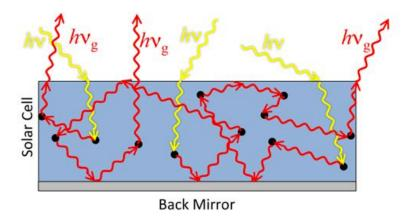
Figure 2.4: Diagram of the case of a solar cell on a perfectly reflecting back mirror; in this case, at open circuit, all the incident photons are absorbed and eventually emitted out of the front surface.
