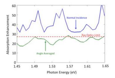
Figure 4.13: The absorption enhancement for the texture in Fig. 4.11, plotted as a function of frequency at normal incidence (blue) and angle averaged (green).
