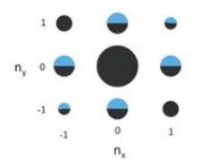
Figure 4.22: The reciprocal space representation for the texture with broken mirror symmetry in Fig. 4.21. The blue pie slices represent the phase of the complex exponential Fourier coefficients.
