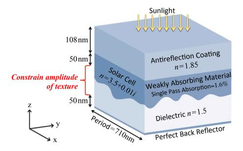
Figure 4.32: Setup for texture optimization with a height amplitude constraint.
