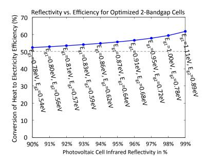
Figure 5.10: The efficiency as a function of photovoltaic cell infrared reflectivity for dual junction cells.  $E_{g1}$  is the bandgap of the top cell in the dual junction stack, and  $E_{g2}$  is the bandgap of the bottom cell. The source radiation temperature is 1500°C, the cell temperature is 20°C, and for both top and bottom cells,  $\eta_{ext} = 0.3$ .
