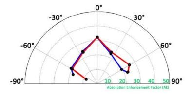
Figure 4.18: The absorption enhancement factor (AE) averaged over frequency and polarization, as a function of incident angle  $\theta$  in the xz plane (blue) and the yz plane (red).
