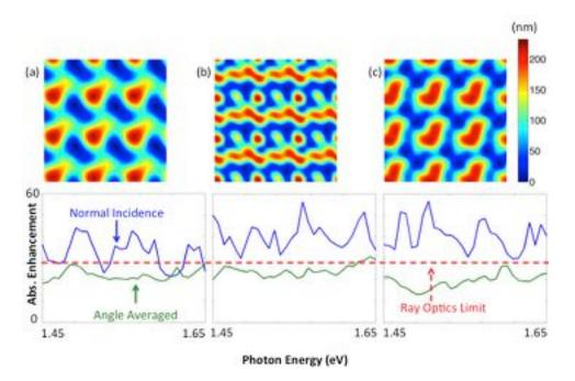
Figure 4.15: The surface textures and absorption enhancement as a function of frequency for different initial conditions, revealing a broad optimum.
