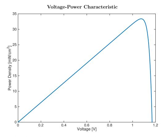
Figure 2.2: The relationship between power and voltage. We use a maximum power point tracker (MPPT) to continually operate the cell at the maximum power point voltage.
