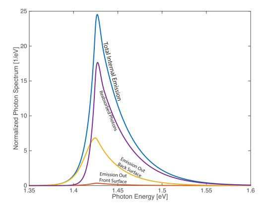
Figure 2.5: The breakdown of internal photons in a GaAs cell, grown on a substrate for a 1 um thick cell. The spectrum is shown for total internal emission, normalized to unity (blue). Of the total internal spectrum, the fraction of photons reabsorbed by the cell (purple), photons escaping out the front surface (red), and photons emitted in the substrate (yellow), are shown.
