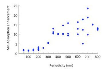
Figure 4.23: Optimizations were carried out at periodicities from 50 to 800 nm, in increments of 50 nm. For each periodicity, at least 3 optimizations were completed for randomly chosen initial starting noise. The Figure of Merit (absorption enhancement for the worst performing frequency and polarization at normal incidence) is plotted for each optimization.
