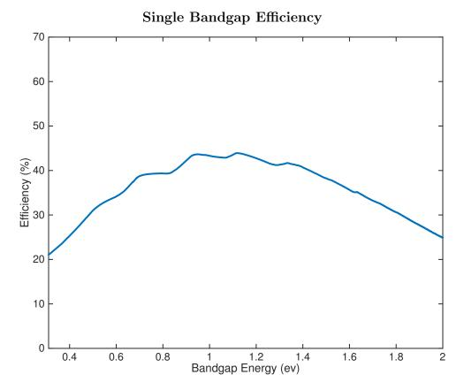
Figure 6.1: Efficiency of single bandgap solar cells under maximum concentration.
