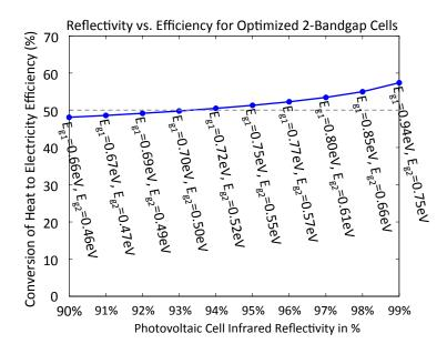
Figure 5.9: The efficiency as a function of photovoltaic cell infrared reflectivity for dual junction cells.  $E_{g1}$  is the bandgap of the top cell in the dual junction stack, and  $E_{g2}$  is the bandgap of the bottom cell. The source radiation temperature is  $1200^{\circ}C$ , the cell temperature is  $20^{\circ}C$ , and for both top and bottom cells,  $\eta_{ext} = 0.3$ .
