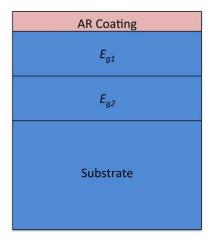
Figure 3.2: Case (1); a dual bandgap solar cell without an intermediate or a back mirror; the top cell, bottom cell, and substrate are index matched with  $n_s = 3.5$ .
