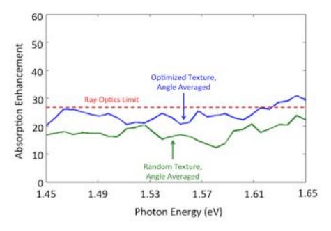
Figure 4.27: The absorption enhancement as a function of frequency, angle averaged, for the optimized texture from Fig. 4.15(b) (blue) compared with the median random texture from Fig. 4.25 (green).
