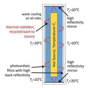
Figure 5.4: Cross-sectional view of the thermophotovoltaic chamber.
