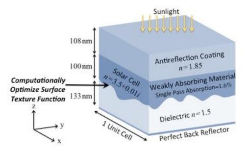
Figure 4.1: The bottom surface texture of the absorbing material is computationally optimized. This diagram is a schematic of 1 unit cell; there are periodic boundary conditions along the yz and xz planes.
