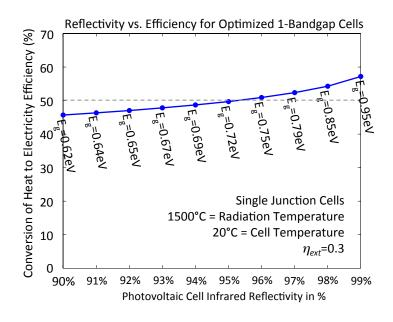
Figure 5.6: The efficiency as a function of photovoltaic cell infrared reflectivity for single junction cells. The source radiation temperature is  $1500^{\circ}C$ , the cell temperature is  $20^{\circ}C$ , and  $\eta_{ext} = 0.3$ .
