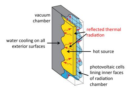
Figure 5.3: Perspective view of the thermophotovoltaic chamber.
