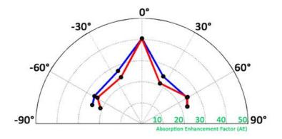
Figure 4.16: The absorption enhancement factor (AE) averaged over frequency and polarization, as a function of incident angle  $\theta$  in the xz plane (blue) and the yz plane (red).
