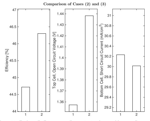
Figure 3.8: Tandem cell efficiency, top cell open circuit voltage, and bottom cell current for bandgaps  $E_{g1} = 1.73$  eV and  $E_{g2} = 0.94$  eV, for Case (2); no intermediate mirror and a perfect back mirror, assuming optically thin cells and Case (3); an air gap intermediate mirror and a perfect back mirror.
