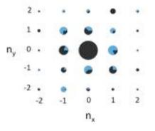
Figure 4.12: The reciprocal (k-) space representation for the final texture seen in Fig. 4.11. The blue pie slices represent the phase of the complex exponential Fourier coefficients.
