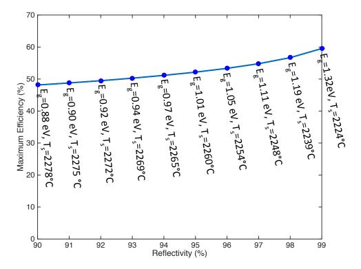
Figure 6.3: Efficiency of solar thermophotovoltaics as a function of back mirror sub-bandgap reflectivity. We denote the temperature of the intermediate layer and the bandgap at each point.
