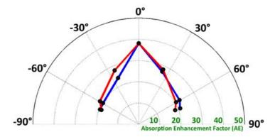
Figure 4.35: The absorption enhancement factor (AE) averaged over frequency and polarization, as a function of incident angle  $\theta$  in the xz plane (blue) and the yz plane (red) for the texture in Fig. 4.33.
