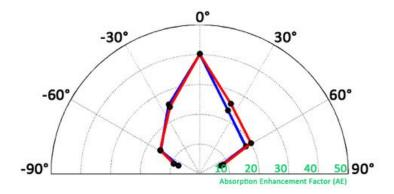
Figure 4.17: The absorption enhancement factor (AE) averaged over frequency and polarization, as a function of incident angle  $\theta$  in the xz plane (blue) and the yz plane (red).
