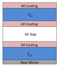
Figure 3.6: Case (3); a dual bandgap solar cell with an air gap intermediate mirror, with perfect antireflection coatings and a perfect back mirror.
