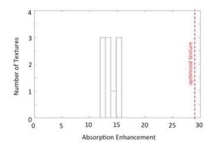
Figure 4.28: The Figure of Merit (minimum absorption enhancement at normal incidence) plotted for 11 randomly generated textures of 2300 nm periodicity. For comparison, the Figure of Merit for the optimized texture in Fig. 4.15(b) is shown by the dotted red line.
