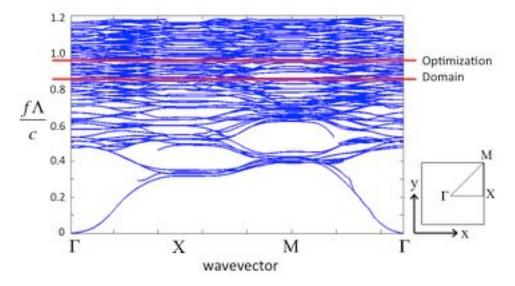
Figure 4.19: The photonic bandstructure for the texture in Fig. 4.15(b).
