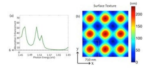
Figure 4.20: (a) The initial absorption enhancement as a function of frequency and (b) a top-down view of the surface texture, for a symmetric texture with a slight perturbation along the diagonal.
