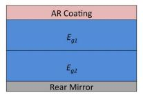
Figure 3.4: Case (2); a dual bandgap solar cell without an intermediate mirror but with a back mirror; the top and bottom cells are index matched with  $n_s = 3.5$ .
