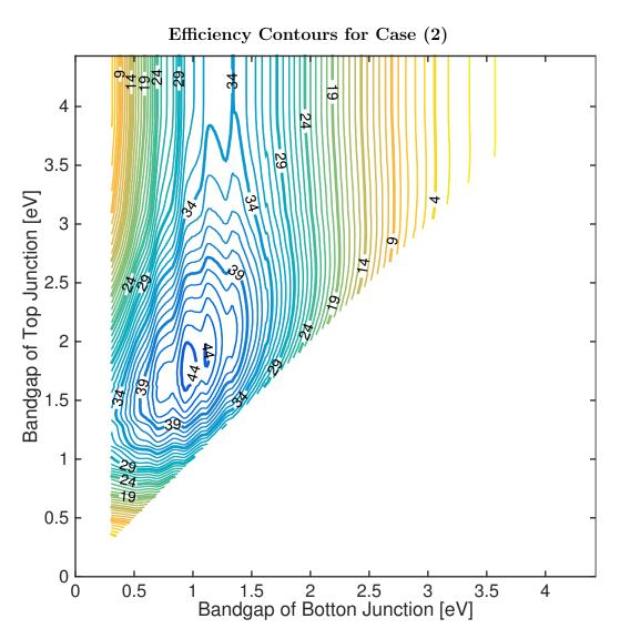
Figure 3.5: The efficiencies as a function of top and bottom bandgap for Case (2), a dual junction solar cell without an intermediate or a back mirror.
