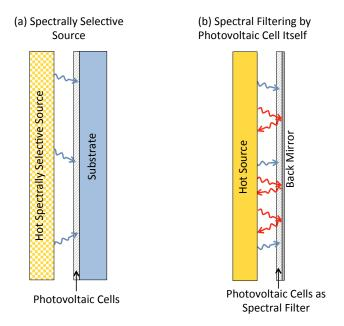
Figure 5.1: For high efficiency, below bandgap photons need to be recycled back to the hot source. This is done with either (a) a spectrally selective source, such as a photonic crystal, which exhibits low emissivity of below bandgap photons (low emissivity of photons is analogous to high reflectivity of photons back to the source) or (b) with a mirror on the back of the photovoltaic cells which reflects the infrared photons back to the source.
