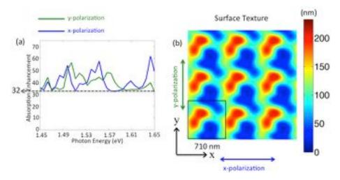
Figure 4.11: (a) The final absorption enhancement as a function of frequency and (b) a top-down view of the surface texture; the colors show the height of the absorbing material (from the antireflection coating to the bottom dielectric, as seen in Fig. 4.1).
