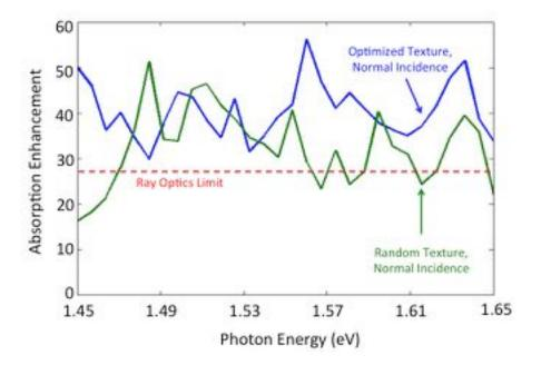
Figure 4.26: The absorption enhancement as a function of frequency at normal incidence for the optimized texture from Fig. 4.15(b) (blue) compared with the median random texture from Fig. 4.25 (green). Lines are averaged over the two orthogonal polarizations.
