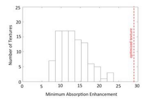
Figure 4.24: The Figure of Merit (minimum absorption enhancement at normal incidence) plotted for 100 randomly generated textures of 710 nm periodicity. For comparison, the Figure of Merit for the optimized texture in Fig. 4.15(b) is shown by the dotted red line.
