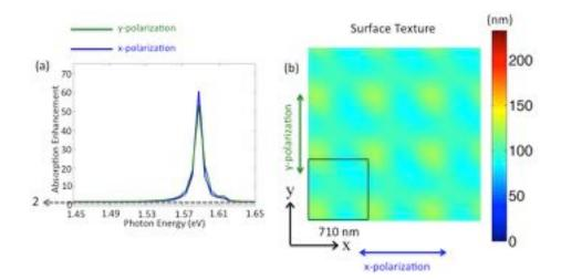
Figure 4.10: (a) The initial absorption enhancement as a function of frequency and (b) a top-down view of the surface texture; the colors show the height of the absorbing material (from the antireflection coating to the bottom dielectric, as seen in Fig. 4.1).
