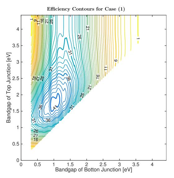
Figure 3.3: The efficiencies as a function of top and bottom bandgap for Case (1), a dual junction solar cell without an intermediate or a back mirror; the cells are assumed to be optically thin to the internally luminescent photons.
