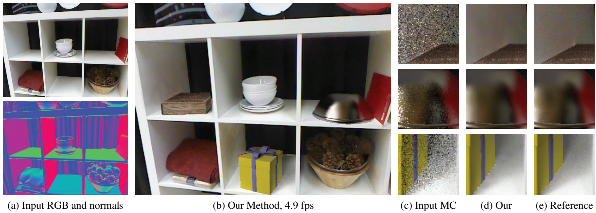
Figure 10: The SHELF scene input image and 3D reconstruction are shown in (a). We insert a diffuse gift-box and a book, and a glossy bowl, as shown in (b). We compare our result (16 spp, 0.20 sec) with unfiltered Monte Carlo (16 spp), which is very noisy, as well as reference (1024 spp, 13 sec) which is 60× slower.
