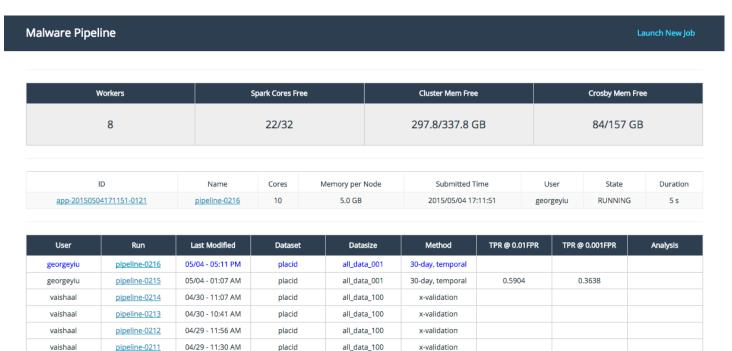
Figure 3: Portion of the pipeline overview page, including cluster status header, running spark job list, and job table.
