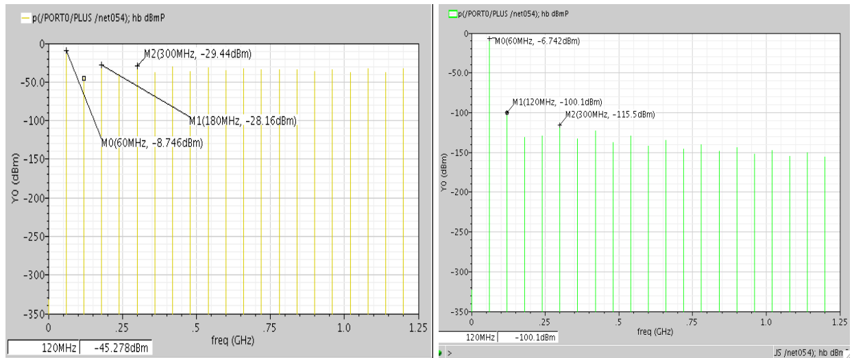
Figure 23: Power without the L-match filtering
