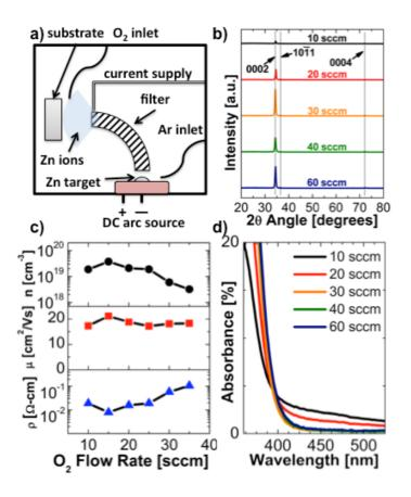
Fig. 2: Cathodic Arc Setup and ZnO Film Characterization (a) Schematic of cathodic arc deposition chamber. The permanent magnet is denoted in red. (b) XRD pattern for ZnO film and varying  $O_2$  flow rates. (c) Electron concentration (n), Hall mobility ( $\mu$ ), and resistivity ( $\rho$ ) as a function of  $O_2$  flow rate. (d) Dependence of optical absorption with  $O_2$  flow rate.
