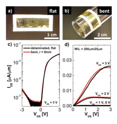
Fig. 4: Flexible TFT Bending Tests Images of the substrate while (a) flat and (b) bent around a test tube with r=8 mm. (c)  $I_{DS}$ - $V_{GS}$  and (d)  $I_{DS}$ - $V_{DS}$  curves for a device on free-standing polyimide with W/L = 200  $\mu$ m/25  $\mu$ m while flat (black) and bent at r=8 mm (red).
