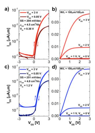
Fig. 3: TFT Performance  $I_{DS}$ - $V_{GS}$  and  $I_{DS}$ - $V_{GS}$  curves for W/L = 100  $\mu$ m/100  $\mu$ m device on (a, b) alkali-free glass and (c, d) polyimide. The arrows on the transfer curves indicate the direction of the double sweep measurement.
