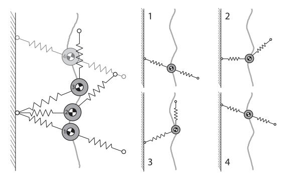
Figure 2.5: A stride of the SLAP model climbing a vertical surface ( $\gamma = 0$ ). (1) The system at touchdown. (2) The system at mid-stance. The unloaded foot continues to follow the prescribed foot trajectory while the foot in stance deflects under load. (3) The system at liftoff. The loaded foot has continued to deflect during stance. (4) The system at the next touchdown. The system is in an aerial phase between (3) and (4).
