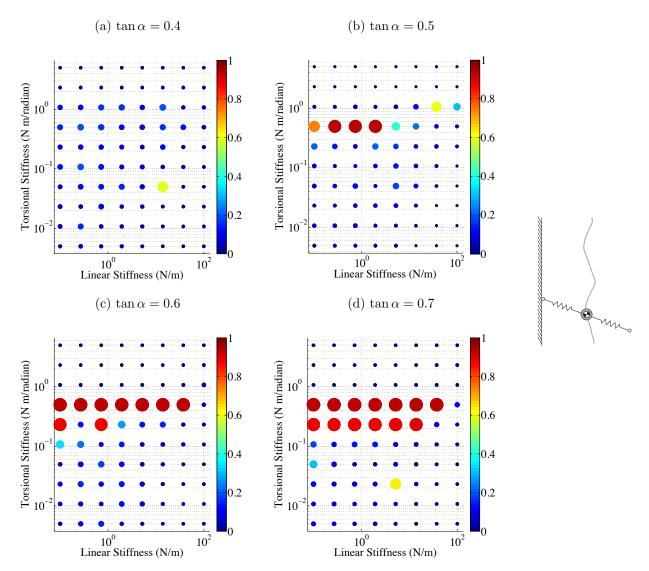
Figure 2.12: A comparison of the performance of the SLAP model on a vertical surface as the shear-to-normal ratio defined by  $\tan \alpha$  is increased for  $\dot{\theta}$ . Velocities are normalized by the product of the angular velocity of the legs and the leg length. Larger, warmer dots indicate a faster normalized average climbing velocity.
