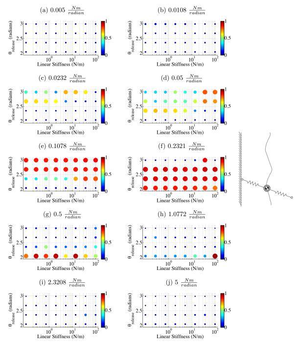
Figure 2.19: Normalized climbing speed of model on a vertical surface with the clock-based controllable adhesive vs. torsional stiffness, linear stiffness, and  $\theta_{release}$ . Velocities are normalized by the product of the angular velocity of the legs and the leg length. Larger, warmer dots indicate a faster normalized average climbing velocity. The stiffnesses in (e) and (g) have large windows of  $\theta_{release}$  which result in effective climbing.
