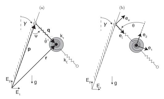
Figure 2.2: Notations used in the SLAP system.
