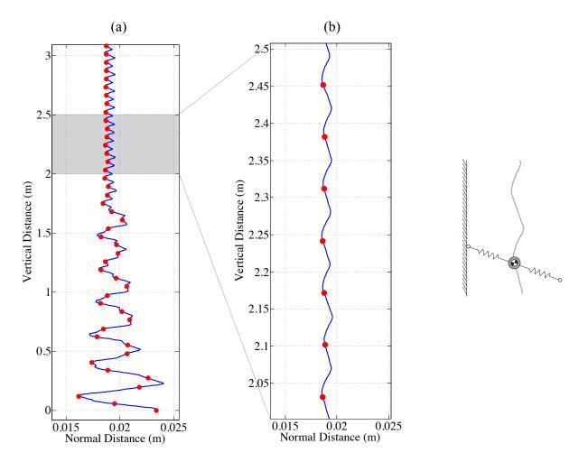
Figure 2.18: The COM translation of the system on a vertical surface with the clock-driven release foot model. The normal axis is magnified to better show normal motion. (a) Initial conditions produce a significant transient in the COM that stabilizes to a periodic gait. (b) Shows a closer view of the COM translations. Red dots show the state of the system at TD events.
