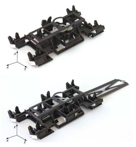
Figure 3.2: CLASH transmission with no legs attached. White leg press-fit connectors allow the legs to be quickly and easily replaced. A tail can be included without modification to the transmission.
