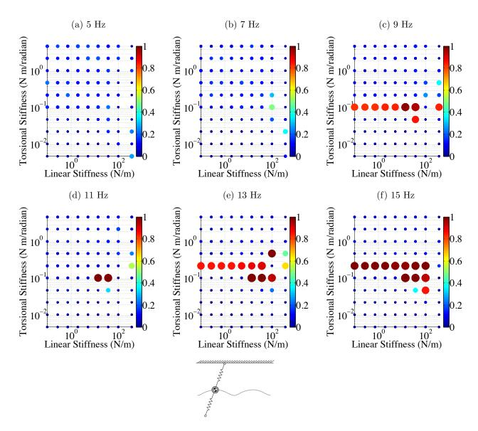
Figure 2.22: Normalized running speed of the SLAP model with the clock-based release foot on an inverted surface with an increased range of possible  $\theta_{release}$ . Velocities are normalized by the product of the angular velocity of the legs and the leg length. Larger, warmer dots indicate a faster normalized average running velocity. With the extended space of  $\theta_{release}$ , the space of linear stiffnesses that result in stable running is increased significantly.
