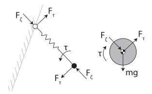
Figure 2.3: Free body diagram of the forces acting on the leg and the COM.
