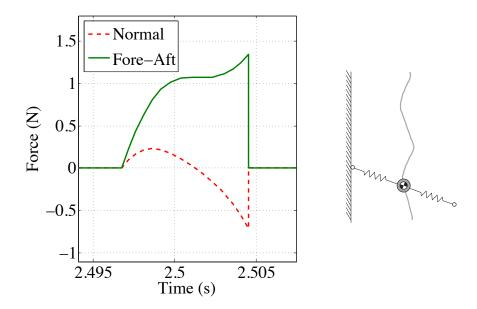
Figure 2.17: Typical ground reaction forces of the model using a controllable adhesive running on a vertical surface. Fore-aft forces are green and normal forces are red. Negative normal forces indicate pulling vertically towards the surface. The initial foot touchdown decelerates the body and accelerates the body away from the surface. Halfway through the stride, the body is accelerated forward and back toward the surface.
