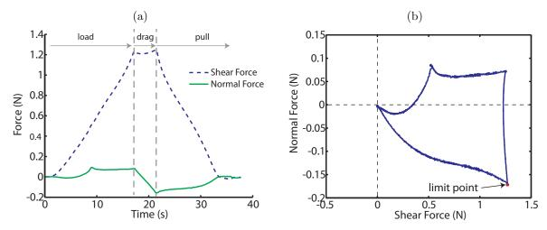
Figure 5.6: (a) Force versus time of the gecko-inspired adhesive foot undergoing a load-drag-pull simulated step at 1 mm/s. (b) The same load-drag-pull step in force space showing the limit point of the gecko-inspired adhesive foot.
