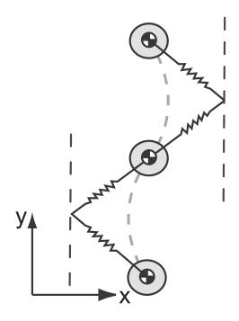
Figure 1.3: Lateral Leg Spring model
