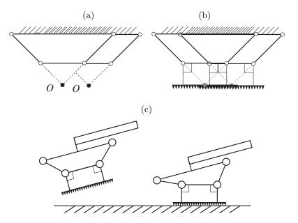
Figure 5.3: (a) The ankle is an isosceles-trapezoid four-bar that creates a remote center-of-motion at O. (b) The remote center-of-motion is designed to be at the bottom of the adhesive. (c) This mechanism allows the foot make coplanar contact with the surface and reduces roll peeling moments.
