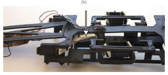
Figure 3.6: Battery placement in CLASH. There is space along the spine of CLASH to house a 60mAh lithium polymer battery to power the system. The battery placement is low and toward the rear of the system to promote a lower pitching moment and passive heading stability. (a) looks at the battery from the side of the system. (b) looks at the battery from the bottom of the robot. Arrows highlight the battery in the structure.
