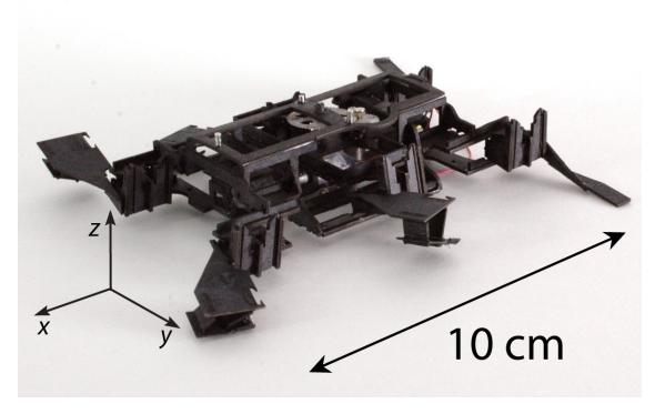
Figure 4.1: CLASH equipped with microspine feet capable of climbing loose and rigidly-backed cloth surfaces.
