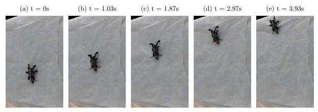
Figure 4.9: A sequence of frames from a video showing CLASH climbing rigidly-backed cloth climbing at approximately 9.5 cm/s.
