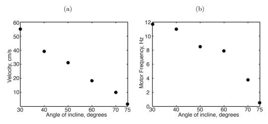
Figure 5.11: (a) The maximum climbing velocity achieved at a given angle of the smooth acrylic above horizontal. (b) The stride frequency of the robot when it was climbing with the maximum achieved velocity.
