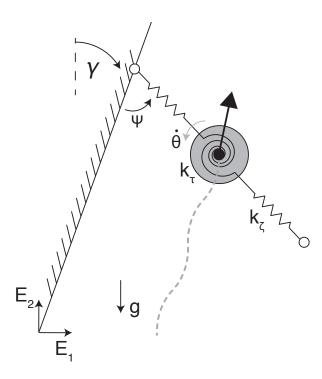
Figure 2.1: Diagram of Spring-Loaded Adhesive Pendulum model
