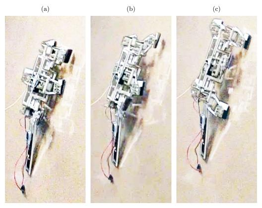
Figure 5.13: Contrast-enhanced frames from high-speed video of CLASH climbing a 70 degree incline at 10 cm second<sup>-1</sup> showing (a) one leg tripod touching the ground, (b) an aerial phase, and (c) the second leg tripod touching down.
