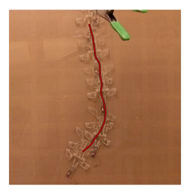
Figure 5.12: Superimposed frames of CLASH climbing a 70 degree incline slope at 10 cm/s. The robot had an initial yaw offset but passively corrected its heading during the climb.
