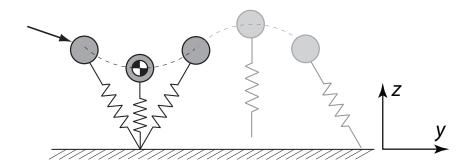
Figure 1.2: Spring-Loaded Inverted Pendulum model
