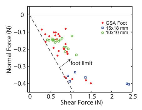
Figure 5.9: A plot of the limit surface of 10x10mm samples (green hollow circle), 15x18mm adhesive samples (blue square) and gecko-inspired adhesive feet (red filled circle).
