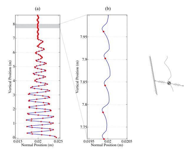
Figure 2.14: The COM translation of the system on a  $\gamma = -5^{\circ}$  surface with the gecko-inspired adhesive foot model. The normal axis is magnified to better show normal motion. (a) Initial conditions produce a significant transient in the COM that stabilizes. (b) Shows a closer view of the COM translations. Red dots show the state of the system at TD events.
