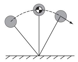
Figure 1.1: Rigid inverted pendulum model
