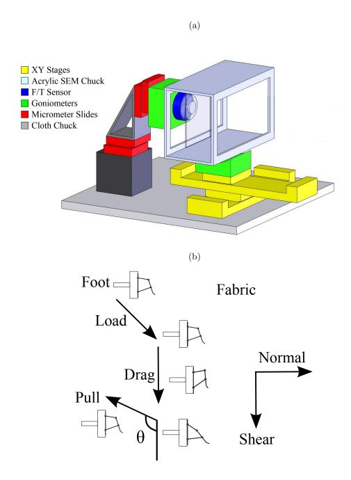
Figure 4.5: (a) The force-displacement apparatus used to test the different foot designs. Feet were mounted on a force sensor and simulated steps were performed on a cloth substrate under displacement control. (b) The simulated step taken by the foot showing the varying pull-off angles that correspond to different running speeds.
