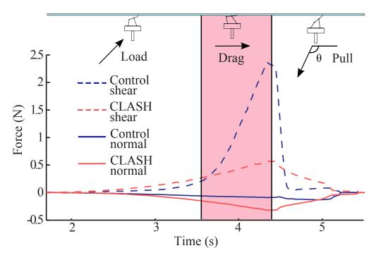
Figure 4.6: An example plot of shear and normal forces during a simulated step for the CLASH and control foot. Note the larger normal engagement force and faster disengagement of the CLASH foot.
