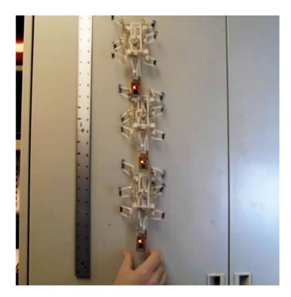
Figure A.2: Superimposed frames of CLASH climbing a vertical metal cabinet at 18 cm second  $^{-1}$ .
