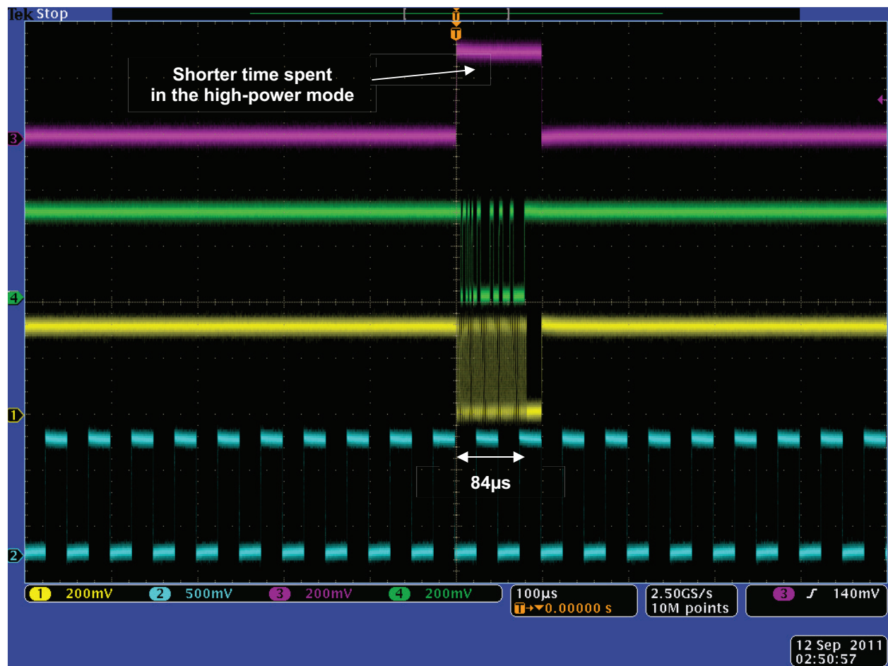
Figure 5.12: Dynamic behavior of asynchronous processor at 0.3V.
