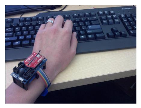
Figure 6.18: Occupant-carried environmental sensing watch
