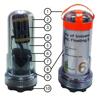
Figure 2.3: Android drifter assembly with part numbers.
