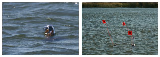
Figure 3.9: Left: drifter under motor power. Right: several drifters participating in experiment.
