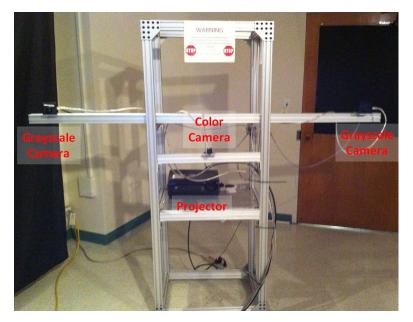
Figure 4.6: Single station from our multi-view structured-light system.
