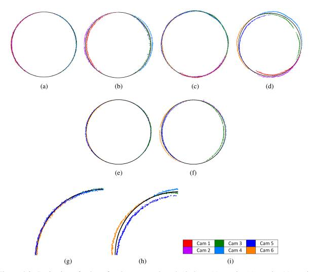
Figure 4.9: Projection of sphere for the proposed method along (a) x-axis, (c) y-axis, (e) z-axis, and for pairwise calibration for (b) x-axis, (d) y-axis, (f) z-axis; (g) zoomed in portion of (a); (h) zoomed in portion of (b). The points for each camera are assigned a unique color (i).
