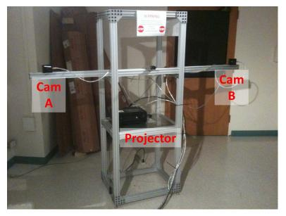
Figure 3.1: Configuration of stereo SL system.
