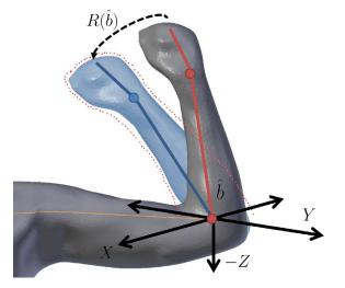
Figure 5.12: An example of branch fitting. The forearm branch of a template is rotated by  $\mathbf{R}(\hat{b})$  to align with points in the target geometry shown as red dots. The new template pose after applying  $\mathbf{R}(\hat{b})$  is shown in blue. The rotation occurs in the world coordinate frame with the origin positioned at the lead joint of the rotating branch.
