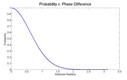
Figure 3.7: Converting absolute phase differences to probabilities.
