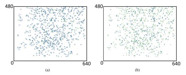
Figure 4.8: Reprojection error using (a) pairwise calibration; (b) proposed method. Image locations are shown in green and the projected image locations in blue.
