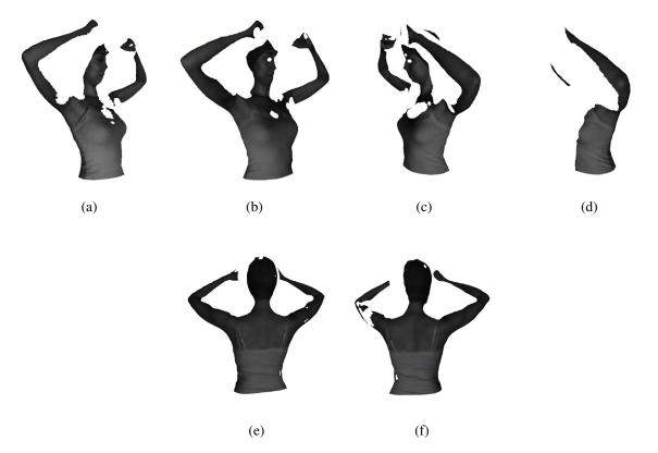
Figure 5.3: Partial meshed point clouds of a human subject generated from unwrapped phase images of a single frame. Views captured from each of the six grayscale cameras in the system: (a)  $C_1$ , (b)  $C_2$ , (c)  $C_3$ , (d)  $C_4$ , (e)  $C_5$ , and (f)  $C_6$  as shown in Fig 5.2.
