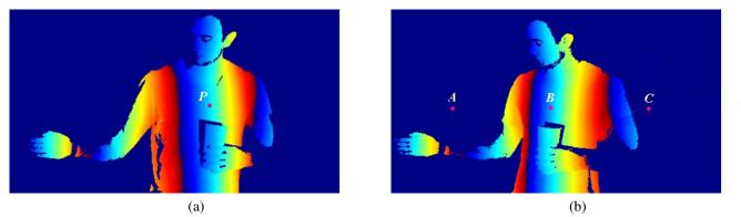
Figure 3.3: (a) Wrapped phase image of the left camera A with the pixel of interest identified by the red dot P; (b) wrapped phase image for the right camera B in a system with the M possible points projected onto the image.
