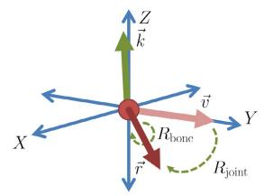
Figure 5.6: An example of the decomposition of  $\mathbf{R}_{\text{local}}$  into  $\mathbf{R}_{\text{joint}}$  and  $\mathbf{R}_{\text{bone}}$ . The original pose of a bone in  $P_0$  always lies along the y-axis with unit vector  $\vec{v}$ . The axis of rotation used to rotate between  $\vec{v}$  and final bone position  $\vec{r}$  is  $\vec{k}$ .
