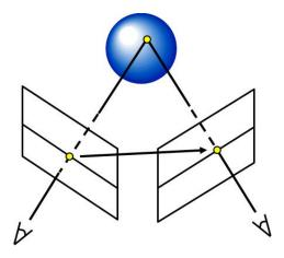
Figure 1.1: Diagram of a simple stereo system.
