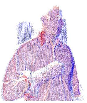
Figure 3.11: Merged camera A (red) and B (blue) points clouds resulting from unwrapped phases of Fig. 3.9.
