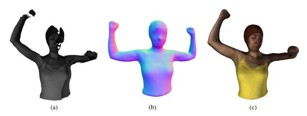
Figure 5.1: Using (a) captured partial scans and (b) a template of a human subject, we generate (c) the time varying geometry of a human subject.
