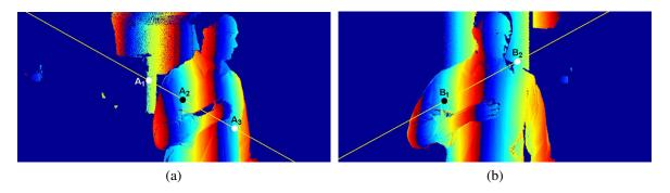
Figure 3.4: Wrapped phase images with epipolar line plotted. Each circle identifies a pixel with the same wrapped phase as the projector pixel; image from (a) camera A; (b) camera B.
