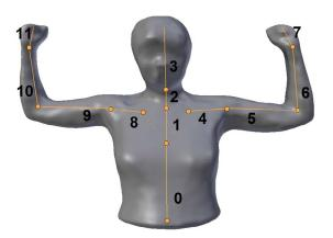
Figure 5.5: Rigged template of a human subject generated by Poisson surface reconstruction. The bones and joints are numbered and indicated in orange.
