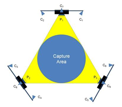
Figure 1.3: Top-down view of the three structured-light stations in our system.
