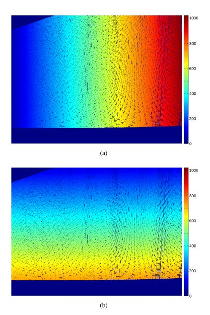
Figure 4.4: Mapping of correspondences from camera c to (a) x-coordinates  $Q_{x:c,p}^t$  and (b) y-coordinates  $Q_{y:c,p}^t$  of projector p.
