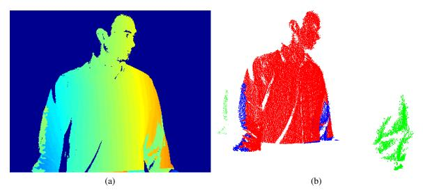
Figure 3.16: Example of 3D geometry from incorrectly unwrapped phase image generated via [91]: (a) incorrectly unwrapped phase image with errors in the arms and bottom of image; (b) resulting geometry; Points in green are due to incorrect unwrapping of some regions in (a); points in blue result from our viewpoint-consistent algorithm which correctly unwrapped those regions.
