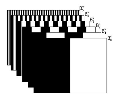
Figure 4.3: Vertical binary-coded projection patterns.
