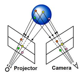
Figure 1.2: Diagram of a simple structured-light system.
