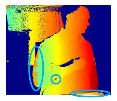
Figure 3.10: Unwrapped image for camera A, corresponding to Fig. 3.4a, using the method in [91]. Erroneous unwrapped regions are circled.
