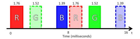
Figure 2.5: The duration of each color channel in a single video frame. The solid bordered color channels represent those that are captured during a single video frame.
