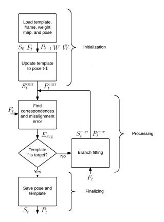
Figure 5.10: Processing steps for the template deformation block shown in Fig. 5.9.
