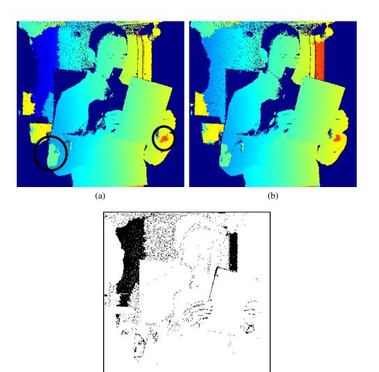
Figure 3.13: (a)-(b) Two successively unwrapped phase images using the method in [91]; (c) regions of phase difference in consecutive images.
