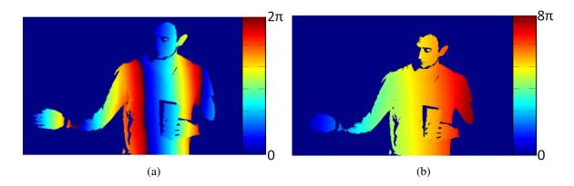
Figure 1.5: An example of a phase image that has (a) wrapped phase values and (b) unwrapped phase values.
