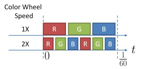
Figure 2.4: Example timings of a  $1 \times vs 2 \times color$  wheel.
