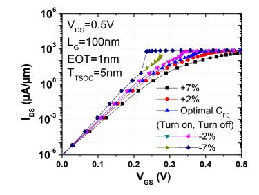
Fig. 3.10 shows that average SS changes almost linearly when  $C_{FE}$  is larger than the optimal value. It also indicates that thicker EOT reduces SS even with  $C_{FE}$  optimized for  $C_{OX}$ . Since  $T_{TSOC}$  and therefore  $C_{DEP}$  is not scaled with  $C_{OX}$  in this case,  $C_{MOS}$  stays in a narrower range from subthreshold to inversion for thicker EOT, resulting in a larger Av (Eq. 1) and therefore smaller SS.
