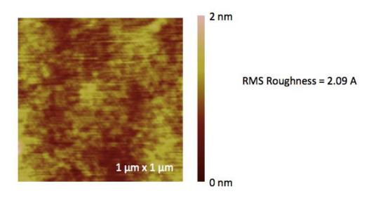
Figure 4.6. AFM topographys of PZT(60nm)STO(8nm)/Si structure
