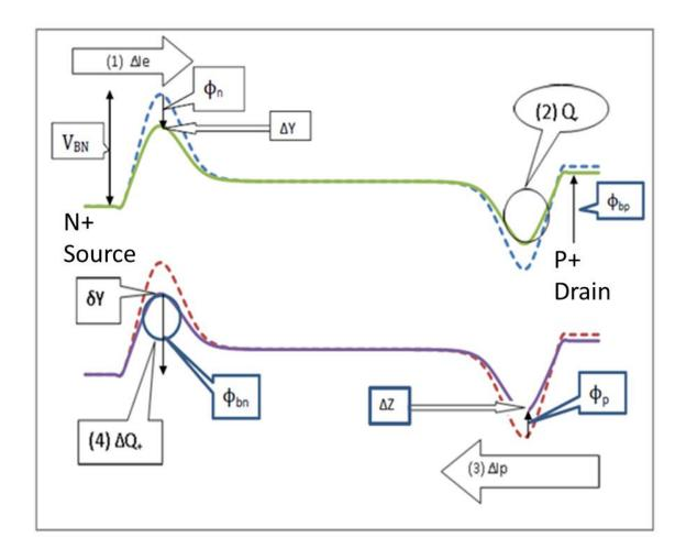
Fig. 2.9: Four steps in the feedback loop. Dash line – Low V<sub>DD</sub>. Solid line – High V<sub>DD</sub>.
