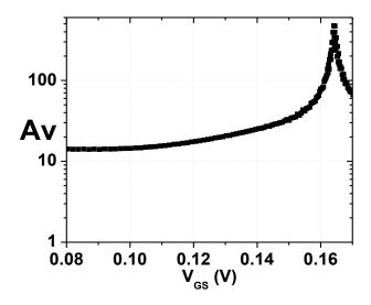
Figure 3.19. Av vs V<sub>G</sub>. Av is extracted from the NCFET ID-VG (VDS=0.5V)
