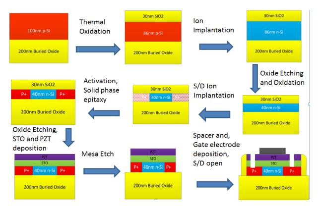
Figure 4.2. Process flow of NCFET fabrication.
