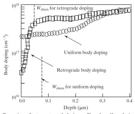
Figure 3.6. Comparison of a steep retrograde doping profile and a uniform doping profile. [3.5]
