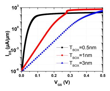
Figure 3.21. Non-hysteretic NCFET ID-VG for different BOX thickness.
