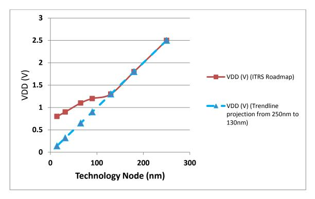
Figure 1.1: Historical trend of V<sub>DD</sub> scaling VS technology node. [1.5]
