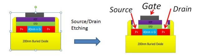
Figure 4.14. Source/Drain contact opening.
