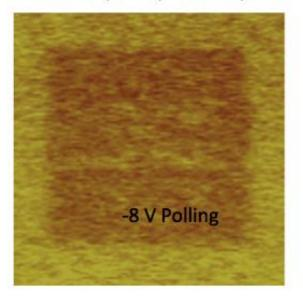
Figure 4.7 Piezo-response force microscopy image of a 1  $\square$ m x 1 $\square$ m region on the surface of the sample.
