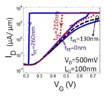
Figure 3.5. Simulated I<sub>D</sub>-V<sub>G</sub> of NCFET with different ferroelectric thickness (t<sub>FE</sub>).
