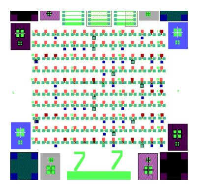
Figure 4.4. Layout of a die.
