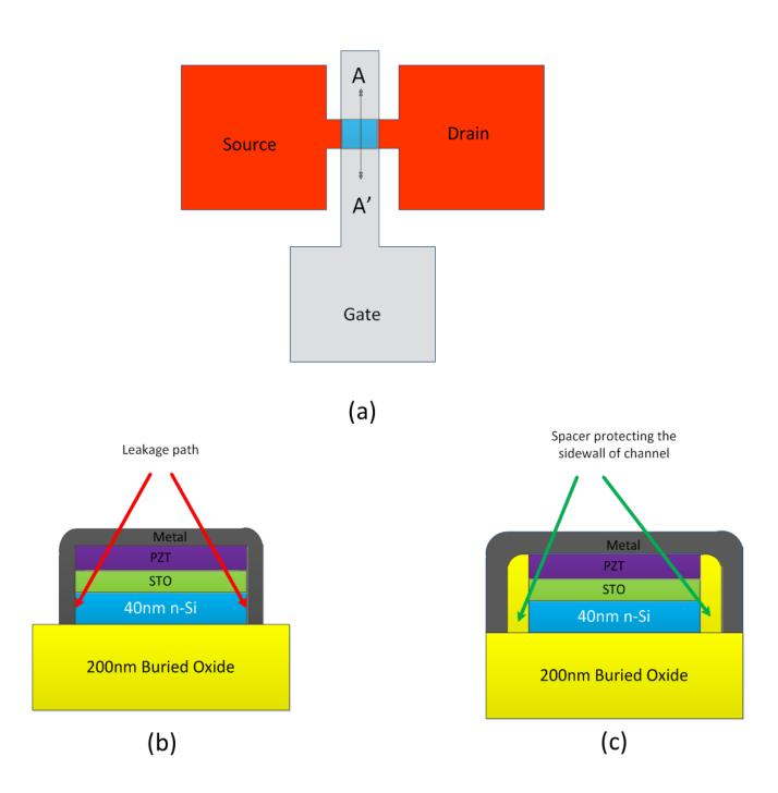
Figure 4.12. (a) Top-down of the device. A-A' indicates the cross-section of (b) and (c). (b) Possible leakage path from gate to channel. (c) Spacer protecting sidewall of the channel.
