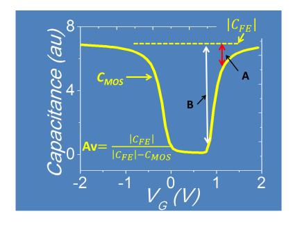
Figure 3.4. Capacitance of  $|C_{MOS}|$  and  $|C_{FE}|$ .
