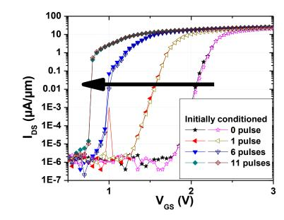
Fig. 2.15. Measured changes in N-FBFET Vt due to N+ side spacer charge reduction. Solid symbols: low Vg to high Vg. Open symbols: high Vg to low Vg. Programmed at Vn=0V, Vp=3V, Vg=-9V. Lg=0.35mm. Vds=0.9V.
