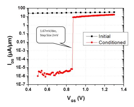
Fig. 2.7: FBFET transistor behavior appears only after properly conditioning the spacer charges.
