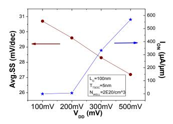
Fig. 3.13 summarizes the I<sub>ON</sub> and average SS at different V<sub>DD</sub>.
