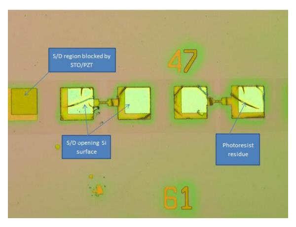
Figure 4.16. Sample after S/D opening (no gate electrode in this sample).
