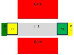
Figure 2.17. Schematic of FBFET structure using ion implantation.
