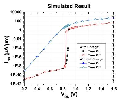
Figure 2.10: Without spacer charge, Id-Vd is that of a PIN diode. After conditioning, steep transition appears. Lg=0.4mm. Vg=0.4V.
