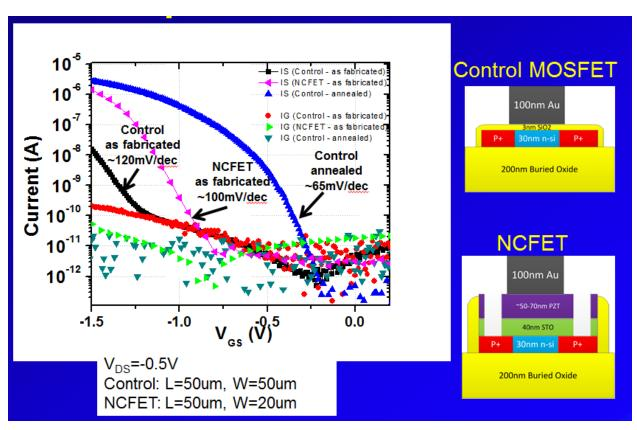
Figure 4.19. Transfer characteristics of pNCFET and control MOSFET.
