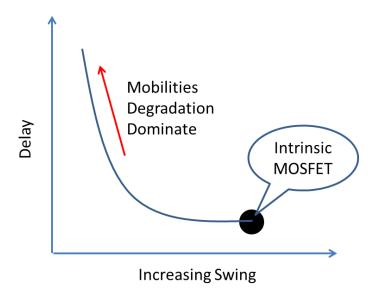
Figure 3.26. Delay vs Swing for NCFET.
