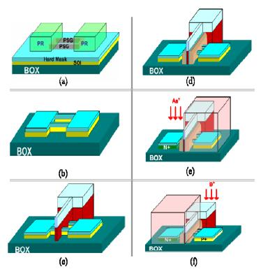
Figure 2.6: Fabrication process flow of FBFET.
