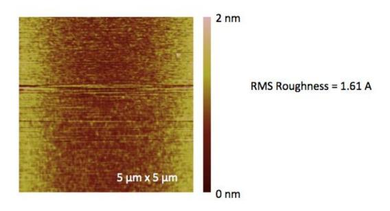
Fig. 4.5. AFM topography of STO/Si structure.
