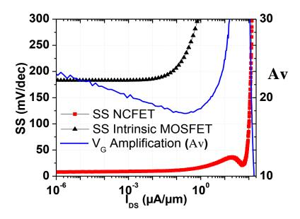
Figure 3.18. Subthreshold Swing and Av VS IDS.
