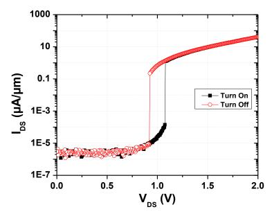
Figure 2.11: Experimental verification of the steep Id-Vd transition. Lg=0.37mm. Vg=-0.5V.
