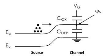
Fig 1.3: Energy Band Diagram from source to channel.
