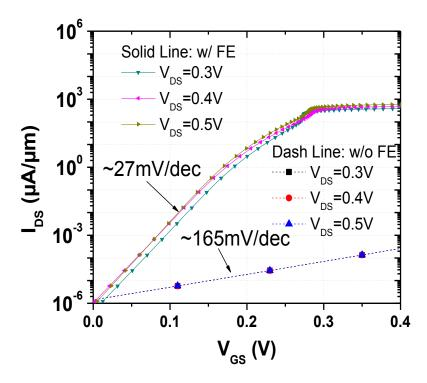
Figure 3.8. 2-D Simulated non-hysteretic NCFET I<sub>D</sub>-V<sub>G</sub> transfer characteristic.
