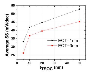
Fig. 3.12. Effects of t<sub>TSOC</sub> and EOT on SS.
