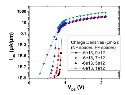
Fig. 2.12 Simulated effects of reducing the P+ side spacer charge. Vn= Vs=0V, Vg=0.4V. Lg=0.4mm.
