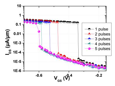
Fig. 2.14 Measured changes in P-FBFET Vt due to P+ side spacer charge increase. Programmed with 10us pulses at Vp=0V,Vn=-8V, Vg=-9V. Lg=0.37mm. Vds=0.9V.
