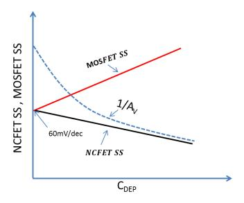
Figure 3.24. Swing vs Depletion Capacitance.
