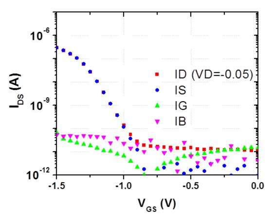
Figure 4.18. I<sub>D</sub>-V<sub>G</sub> of pNCFET.
