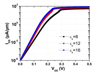
Figure 3.22 Non-hysteretic NCFET ID-VG for different dielectric constant body material.
