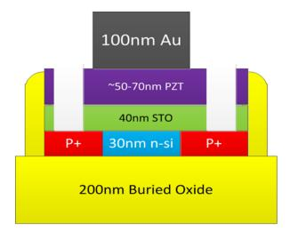
Figure 4.17. Schematic of fabricated pNCFET structure.
