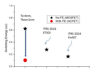
Figure 2.28. Simulated switching energy and ITRS roadmap for ETSOI and FinFET.
