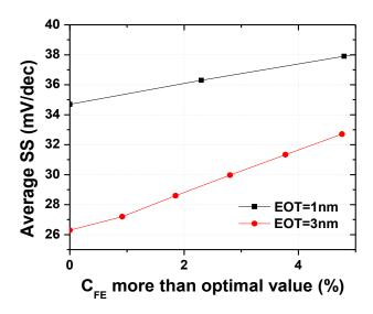
Figure 3.10. Effects of C<sub>FE</sub> larger than the optimal value
