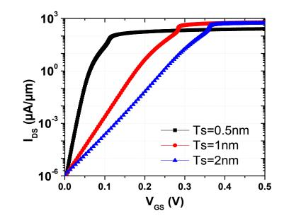
Figure 3.20. Non-hysteretic NCFET ID-VG for different body thickness.
