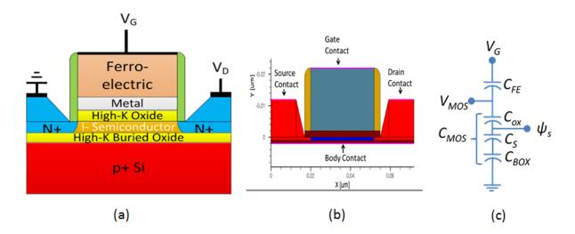
Figure 3.14. (a) Schematic (b) Simulation structure (c) Capacitance Model
