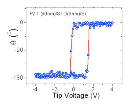
Fig 4.8 Piezo-phase response of the sample as function of the applied voltage.
