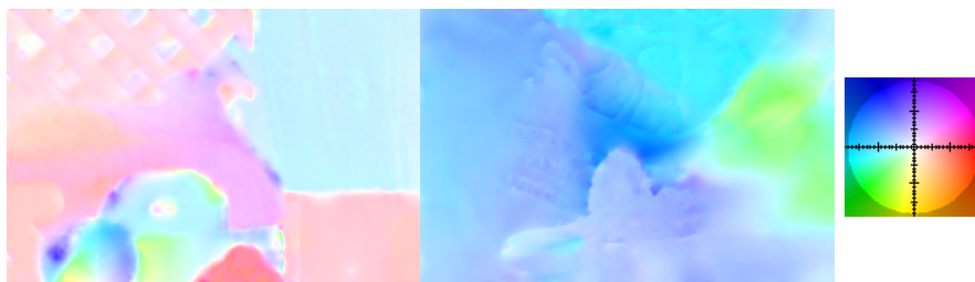
Figure 7.4: Visualization of flow field, produced using the Middlebury visualization tools [123], resulting from multi-level Horn-Schunck with median filtering. Two benchmark images are shown: RubberWhale and Dimetrodon. The color code on the right maps motion to colors. The colorcode figure is reproduced from Baker et al [123].
