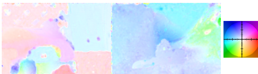
Figure 7.4: Visualization of flow field, produced using the Middlebury visualization tools [123], resulting from multi-level Horn-Schunck with median filtering. Two benchmark images are shown: RubberWhale and Dimetrodon. The color code on the right maps motion to colors. The colorcode figure is reproduced from Baker et al [123].
