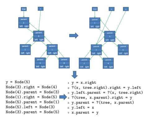
Figure 2.4: The first trace of a left rotation of a binary tree. The user is shown the left tree and manipulates it to reach the right tree.
