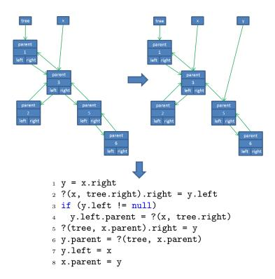
Figure 2.5: The second trace of a left rotation of a binary tree. The user is shown the left tree and manipulates it to reach the right tree.
