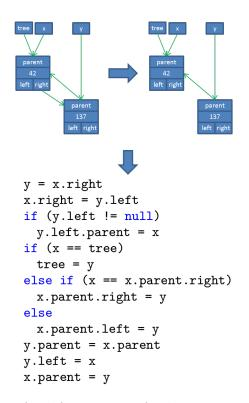
Figure 2.7: The fourth trace of a left rotation of a binary tree. The user is shown the left tree and manipulates it to reach the right tree.
