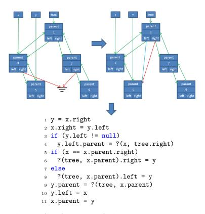
Figure 2.6: The third trace of a left rotation of a binary tree. The user is shown the left tree and manipulates it to reach the right tree. The red arrows represent the choices our tool shows the user and the blue arrows are the correct changes.
