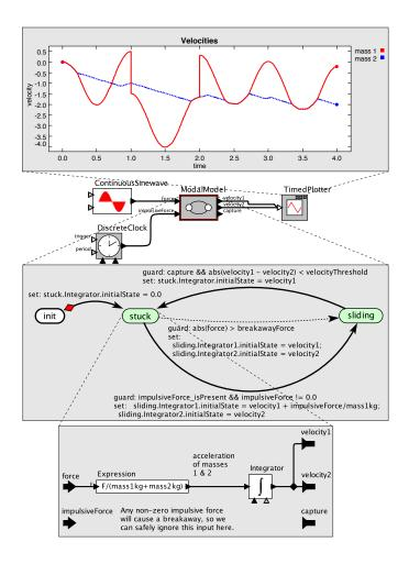
Fig. 29. Model of friction with impulsive collisions. [online]
