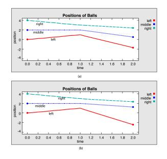
**Fig. 14.** (a) Interleaving of simultaneous impulsive forces where the collision of the left ball (with mass 0.2kg) with the middle ball (with mass 1kg) is handled before the collision of the right ball (with mass 5kg) with the middle ball. [online] (b) Interleaving the collisions in the opposite order yields different behavior. [online]
