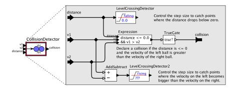
Fig. 10. A Ptolemy II model of a collision detector.
