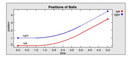
**Fig. 15.** Positions of two balls that start out touching and not moving. From time 1, a constant force is applied to the left ball, which results in pushing both balls to the right. At time 3.5, we stop applying the force, so the balls drift together at the same velocity. [online]
