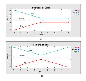
**Fig. 12.** (a) Superposition of simultaneous impulsive forces results in instant loss of energy. [online] (b) Interleaving of simultaneous collisions at distinct microsteps conserves energy. [online]
