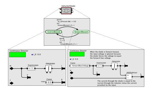
Fig. 38. Implementation of the InductorDiode in Figure 36.
