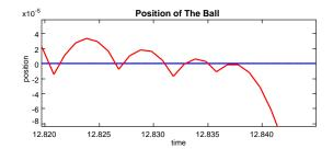
**Fig. 21.** Detail of the point in simulation where the bouncing ball tunnels through the surface.
