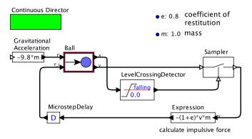
Fig. 18. Bouncing ball using impulsive forces. [online]
