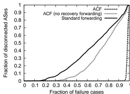
Figure 2: Prevalence of transient disconnection after a single provider link failure. The x-axis represents the fraction of all failure cases that cause some disconnectivity with traditional forwarding.
