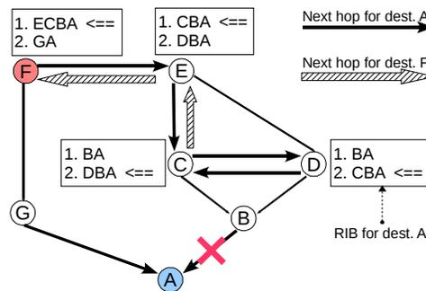
Figure 1: A sample AS-level topology with a transient forwarding loop.
