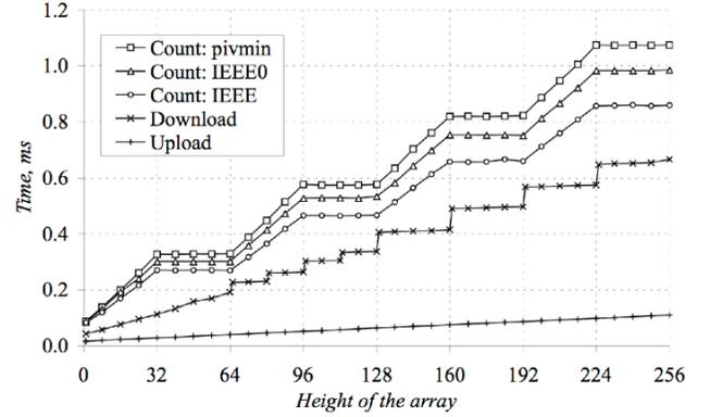
Figure 4: Running times of different GPU stages and versions of  $Count(x)$  for  $n = 192$ . Upload is the transfer to the GPU memory, and download is other way around. For height  $H$ ,  $256 \times H$  instances of  $Count(x)$  are run.
