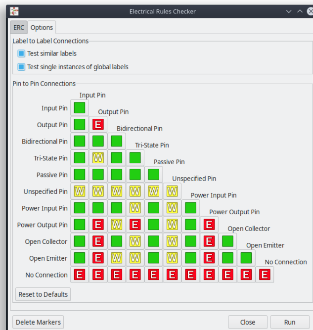
Figure 1.4: An electrical rules checking (ERC) pin compatibility matrix. Schematic capture tools try to provide error checking by assigning schematic pins to a small set of classes and using a matrix, like the one shown, to determine whether each connection is valid. Schematic editors lack the information needed for more substantive checks. This simplified model creates many false positives and false negatives.
