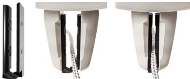
Figure 3.3: Pinch-Cage (PC) Jaws . Left: a rendering of the design of the pinch-cage gripper jaws, which attach to the YuMi’s standard white gripper. Center: the cage grasp, in which the perpendicular “foot” segment of the attachment enables the cable to slide freely. Right: the pinch grasp, in which the cable is held tightly, preventing slack from slipping through.
