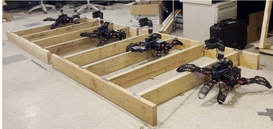
Figure 1.3: Time-lapse photo capturing the SpiderPi robot climbing over 8 joists using the method proposed in our work.
