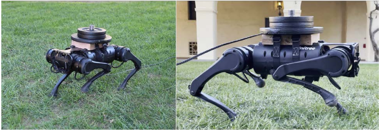
Figure 5.1: The 12 kg A1 robot carrying 10 kg of payload with our method, tested for trotting in place and walking forward.
