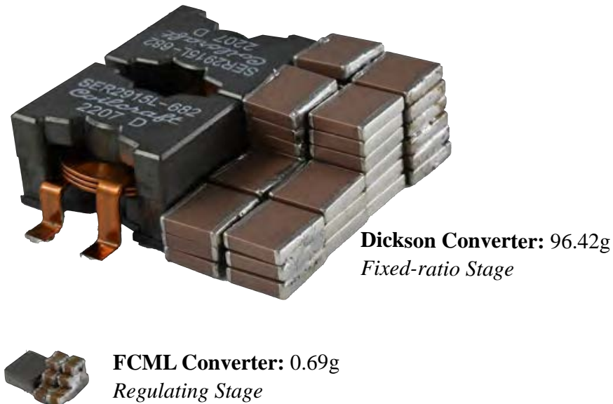
Figure 9.16: Photograph of passive components utilized in the hardware prototype. Components are chosen to minimize total passive mass in the Dickson converter and FCML converter. The passive components are shown in the same scale, and highlights the small volume and weight of the FCML converter which is designed to process minimal power.
