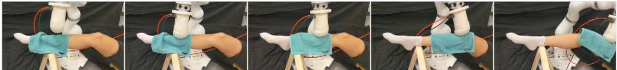
Figure 4.9: The robot cleans the the length of a leg with a damp washcloth and maintains constant contact even over the knee. ©2022 IEEE.
