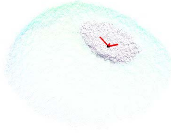
Figure 5.2: Example point cloud reading of the tactile sensor, with black deformed portion and red principal component vectors. ©2020 IEEE.
