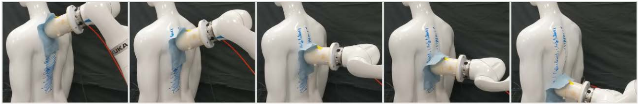
Figure 4.12: The robot cleans down the length of a mannequin’s back. ©2022 IEEE.
