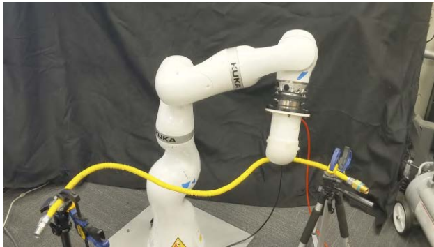
Figure 5.1: Geometric tactile features for interaction-based tasks, eg. edge-following, cannot be encoded by wrench signals. ©2020 IEEE.
