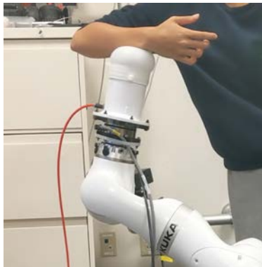
Figure 3.1: The proposed soft interface enables safe and precise tactile interaction between a human and a robot. ©2020 IEEE.
