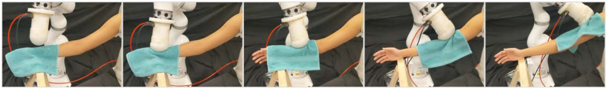
Figure 4.8: The robot wipes along the length of an arm with a damp washcloth, cleaning away a trail of black pepper. ©2022 IEEE.
