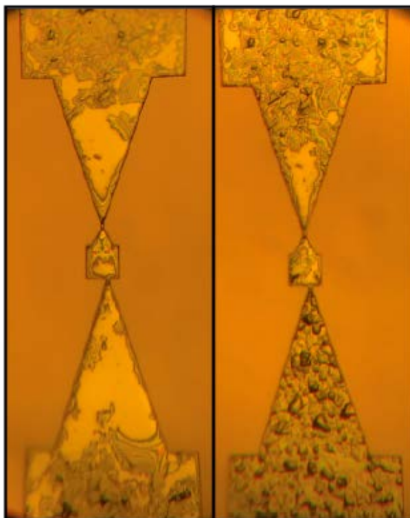
Figure 4.4: Spin coating multiple coats of hydrogel blend increases volume of dried hydrogel deposited in chambers. Left: single coating of hydrogel blend after dehydration. Right: triple coating of hydrogel blend after dehydration.
