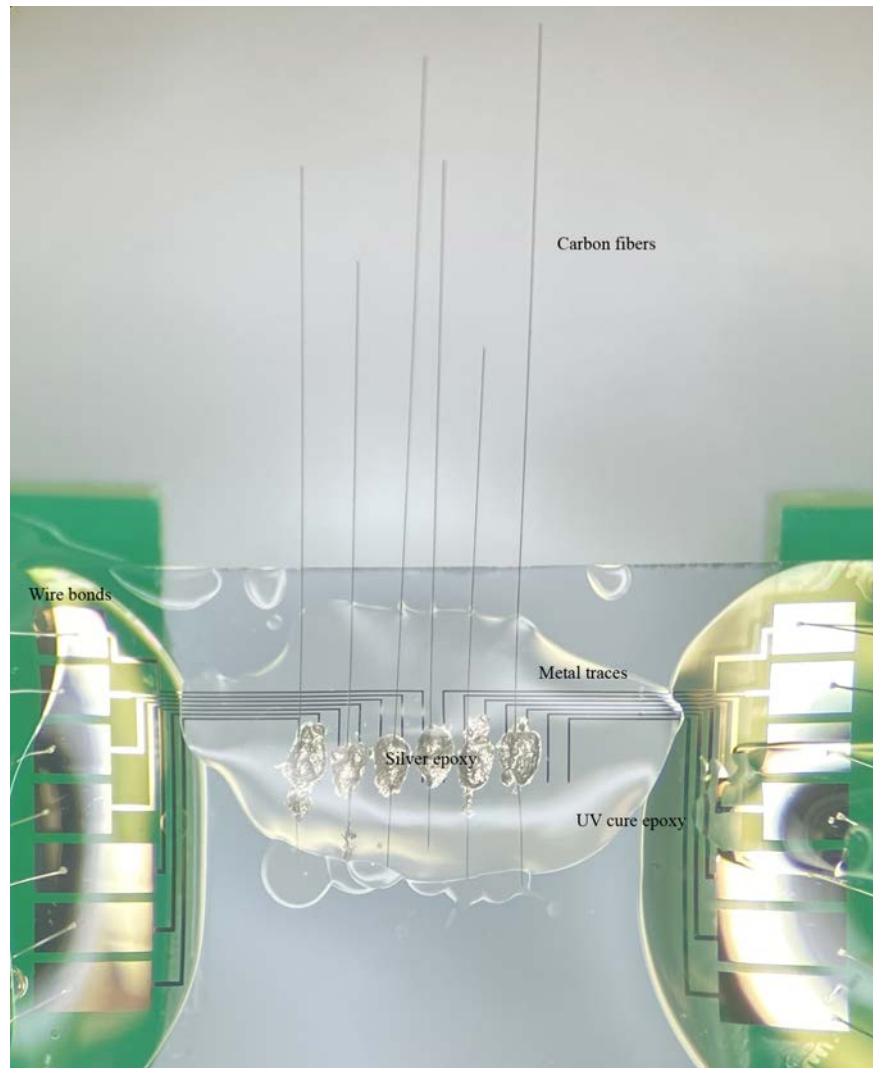
Figure 3.4: Fibers are shorted to PCB pads via microfabricated breakout board and silver epoxy. UV cure epoxy is used to electrically insulate the traces and silver epoxy.
