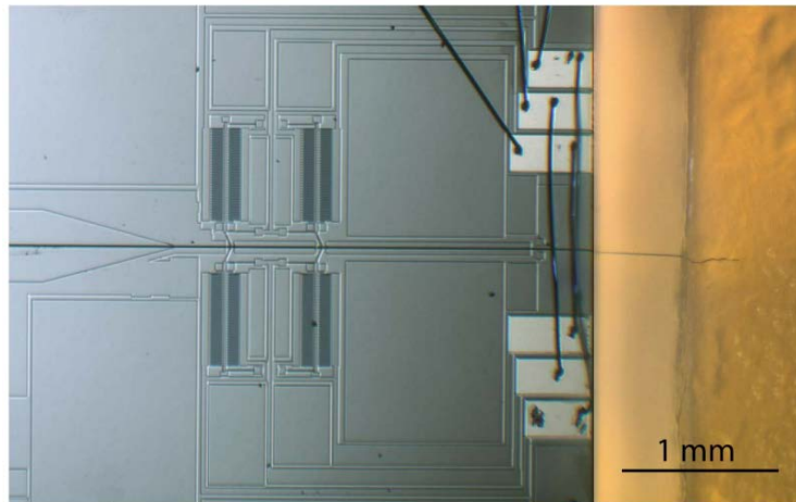
Figure 1.11: Electrostatic MEMS inchworm actuator inserting a carbon fiber into brain phantom. Reproduced from [93] with permission.
